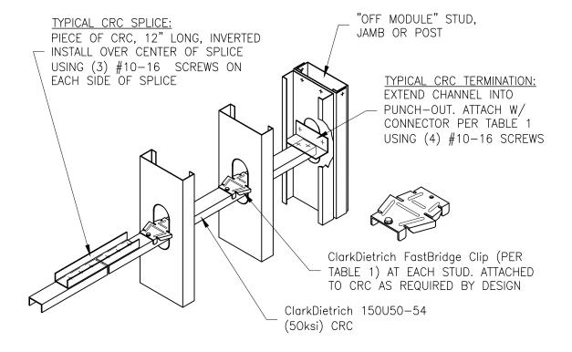
THIS DETAIL IS NOT SUITABLE FOR WALL STUDS DEEPER THAN 8"
