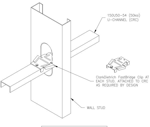
THIS DETAIL IS NOT SUITABLE FOR WALL STUDS DEEPER THAN 6"
