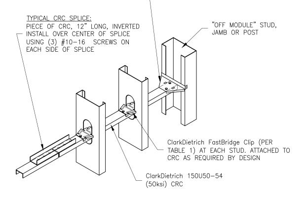
THIS DETAIL IS NOT SUITABLE FOR WALL STUDS DEEPER THAN 6"
