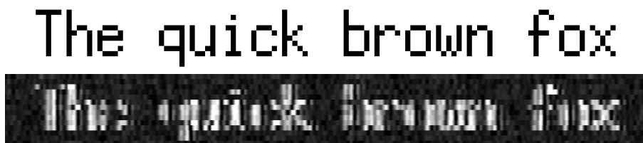
Figure 2: Text displayed on a cathode-ray tube (top) and signal seen by eavesdropper (bottom).
