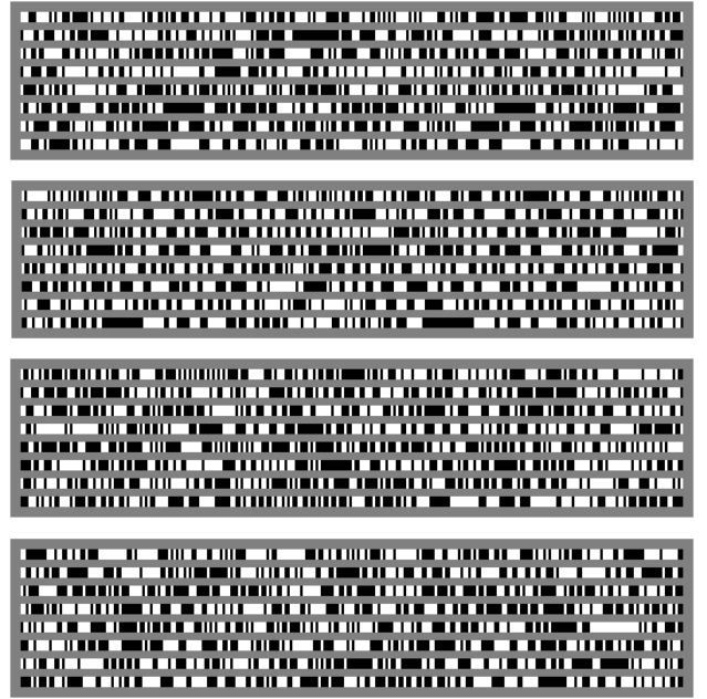
Fig. 1. Representation of the IrisCodes [10] produced by four different eyes. The eight rows within each can be regarded as eight concentric rings, each encoding a [0, 2\pi] traversal around the iris. (Eyelid masking is not shown.)
