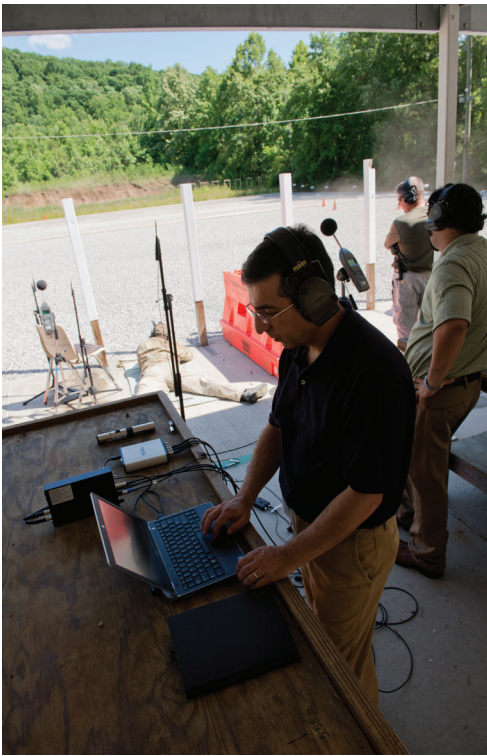
Figure 2. NIOSH investigator acquiring and analyzing impulsive noise data on laptop computer using NIOSH Impulsive Measurement System. Photo by HHE requestor.
