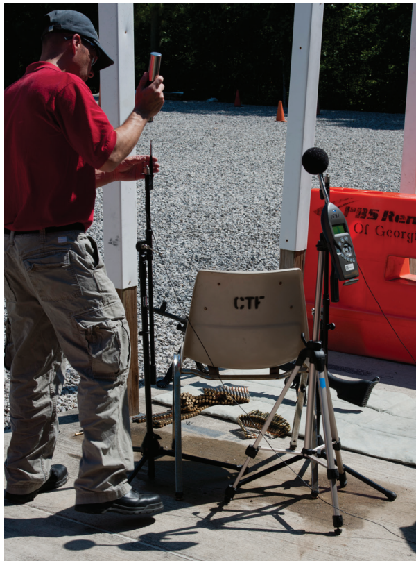
Figure 1. NIOSH investigator positioning and calibrating a one-eighth inch microphone for impulsive noise measurements. Photo by HHE requestor.
