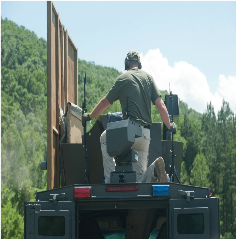
Figure 4. Firing range instructor kneeling between microphones and behind a noise barrier on top of modified SWAT vehicle during firing of Dillon 134D Aero Minigun. Photo by HHE requestor.
