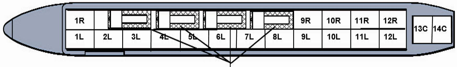
**Loadable locations for engine transport device with MD-11, 767, or 747 engines**
