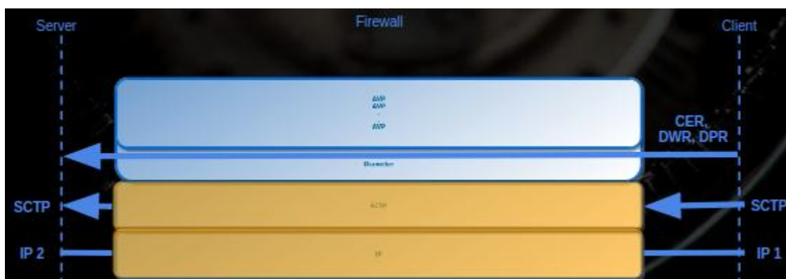
Figure 6.2.1b - Diameter Firewall connections
