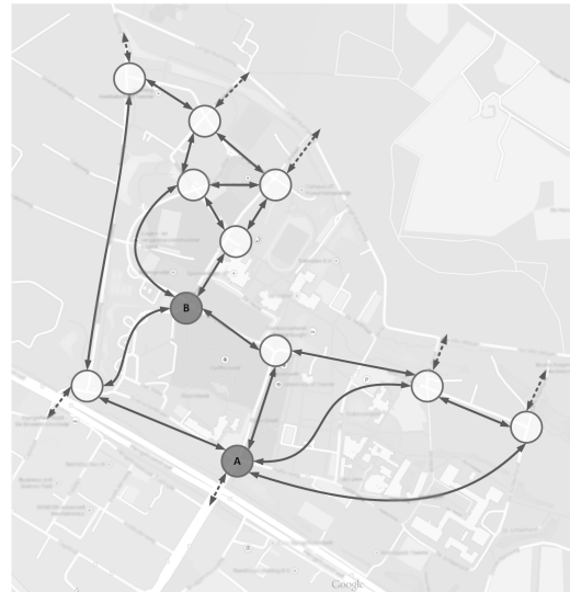
Figure 4: Turning road network into a graph
