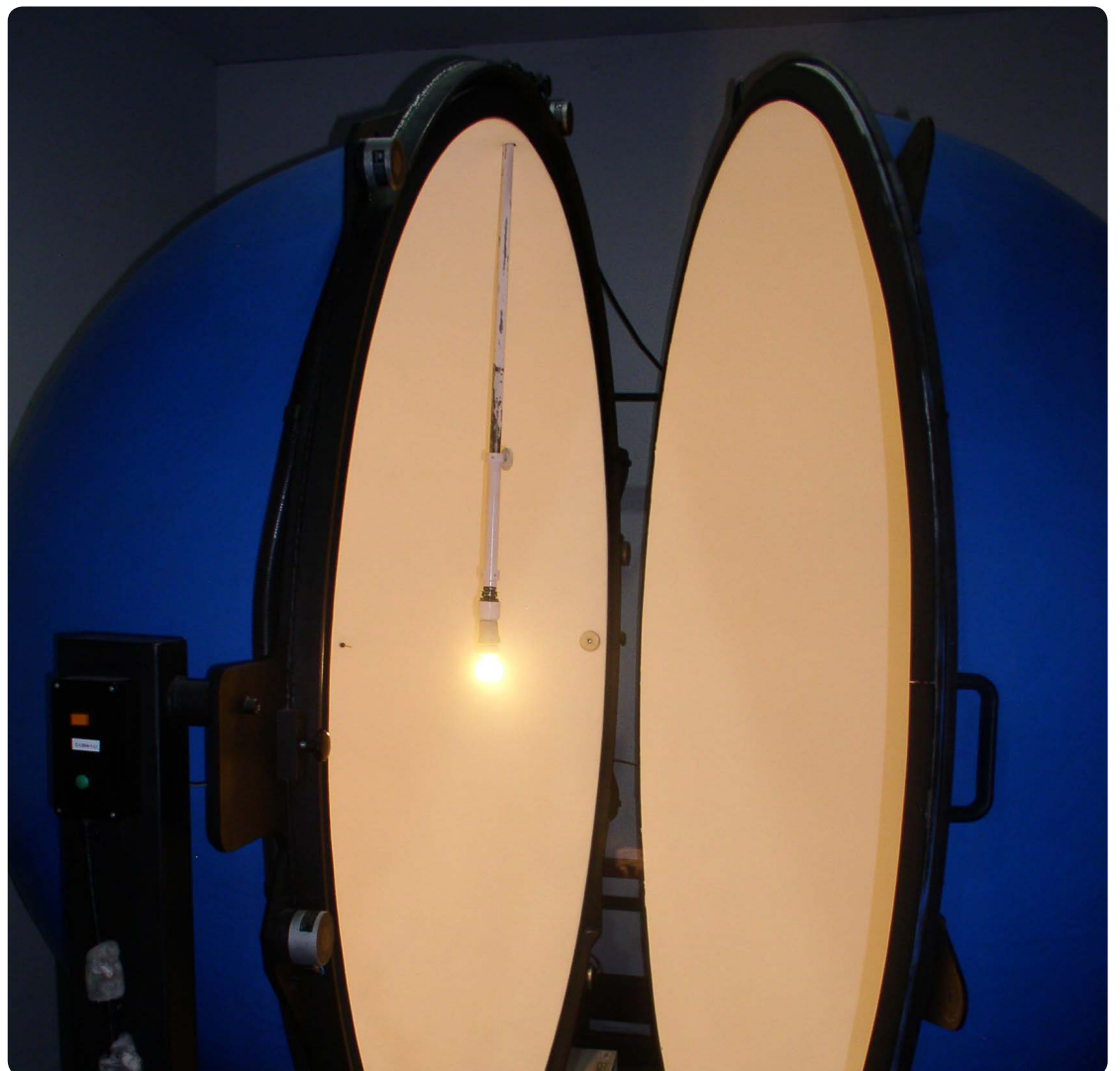
A lightbulb is prepared for luminous flux testing in a spherical chamber that completely closes to eliminate ambient light
