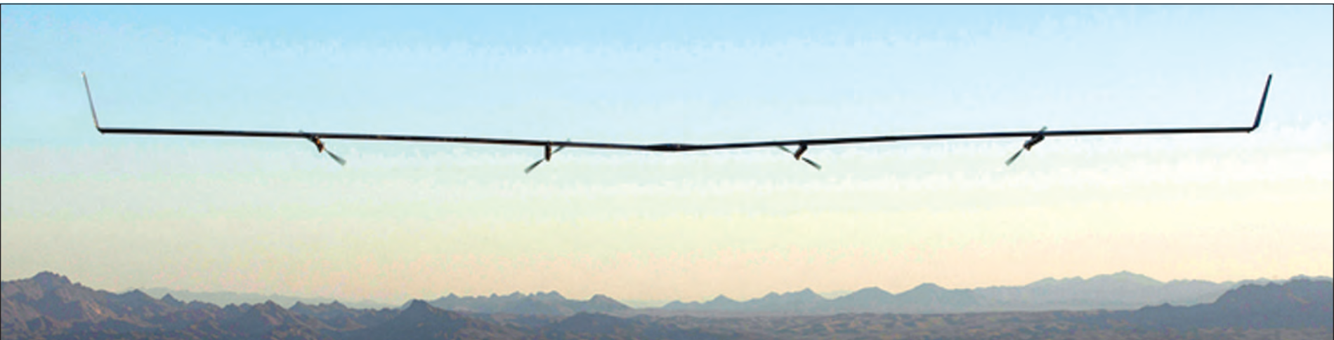
The Aquila UAS will carry a communications payload that will use lasers to transfer data more than 10 times faster than existing systems. It will be able to aim its beams precisely enough to hit a dime more than 11 miles away while in motion.
