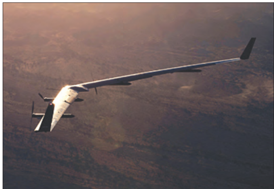
By design, Aquila does nothing fast: It climbs slowly, and descends even slower. The solar-powered craft is extremely efficient, running on the power equivalent of three blow dryers. (Loaned photos)
