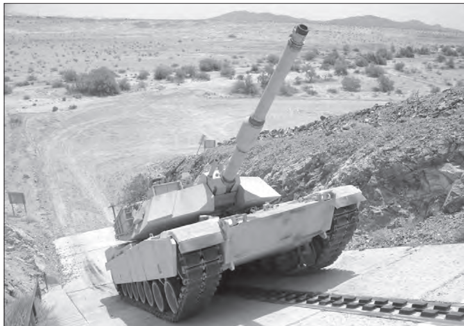
Yuma Proving Ground's Ground Combat Systems Branch puts military vehicles through a grueling reliability and performance regimen in desert terrain. When not racing across scores of miles of hot, treacherous desert road courses, vehicles like this M1 Abrams are put through other stresses, such as climbing this awing 60% grade. In comparison, the steepest grade on an American interstate highway is 6%. (Photo by Mark Schauer)
