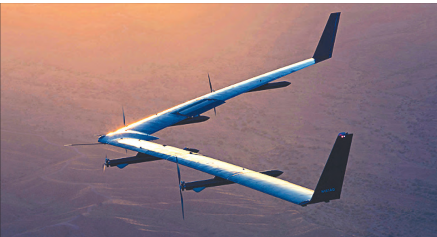
Facebook recently conducted a successful second full-scale test flight of their Aquila unmanned aircraft at YPG. The solar-powered aircraft seeks to beam internet to remote parts of the world and eventually break the record for longest unmanned aircraft flight.
