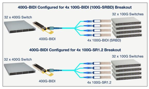
In summary, Arista's 400G-BIDI transceiver is software configurable to operate in any one of three operating modes:
