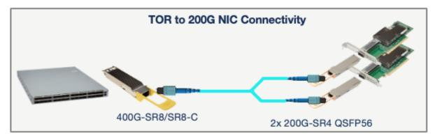
The 400G-SR8-C transceiver has the same features as the 400G-SR8, with the added ability to breakout into 8x 50G-SR or 8x 25G-SR optical links. It can therefore be used in applications that require high density 50G or 25G breakouts – as illustrated below.
