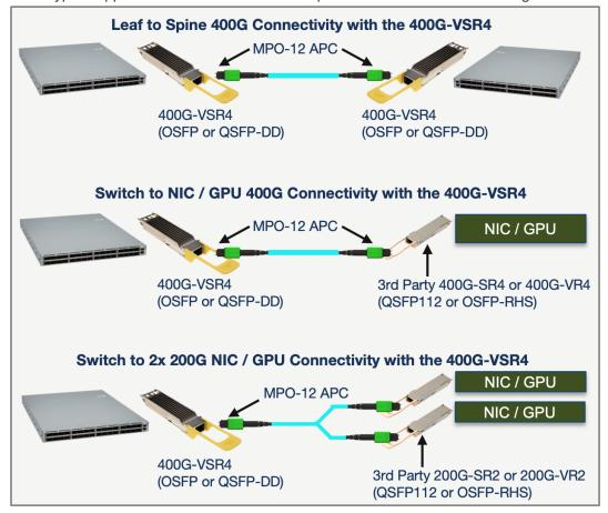
400G-VSR4 transceivers use MPO-12 APC (Angled Physical Contact) fiber connectors to reduce optical back reflectance. Note that all 40G and 100G parallel MMF optics (such as the QSFP-40G-SR4 and QSFP-100G-SR4) use MPO-12 PC/UPC (un-angled) fiber connectors, so care must be taken to ensure that only MPO-12 APC connectors are used with OSFP-400G-VSR4 and QDD-400G-VSR4 modules.
