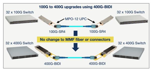
When configured for 400GE operation, the 400G-BIDI transceiver is compliant with the IEEE 400GBASE-SR4.2 specification for 400GE over 4 pairs of MMF.
