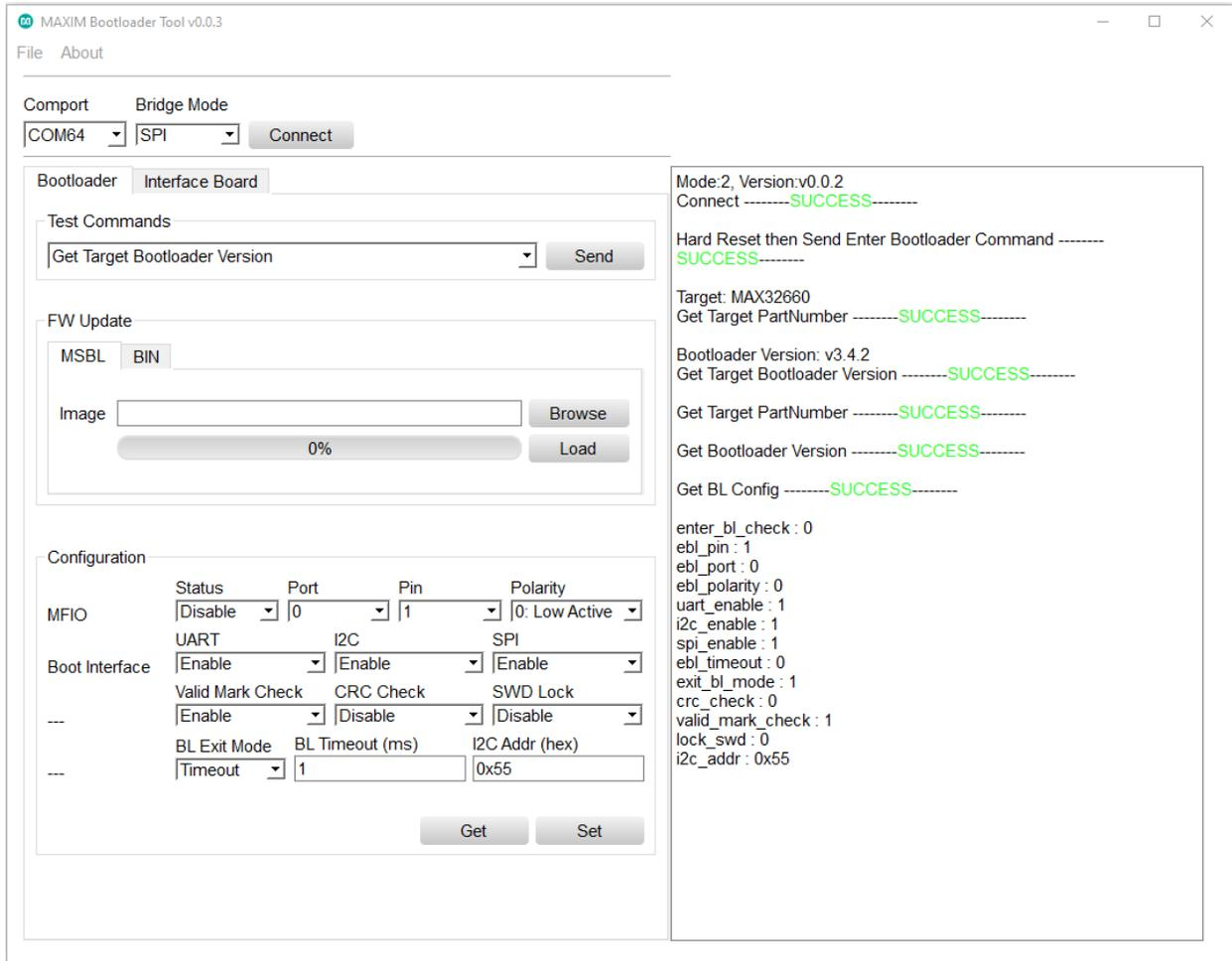
Figure 16. Bootloader GUI tool reading bootloader configuration parameters.
