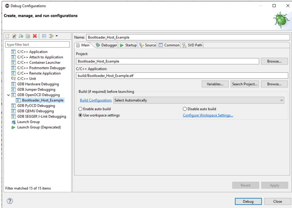
Figure 27. Loading binary on target EV kit.
