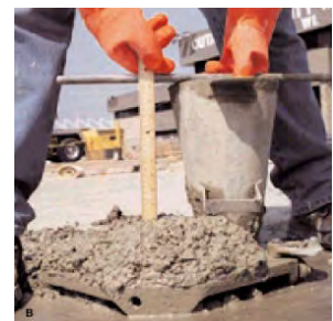
Figure 5 – Concrete mix with high slump
