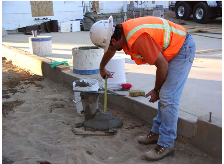
Figure 11 – Performing the slump test in the field
