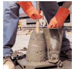
Figure 4 – Concrete mix with low slump
