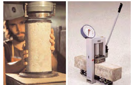
Figure 3 – Testing the concrete cylinder for compressive strength (left) and concrete beam for flexural strength (right)
