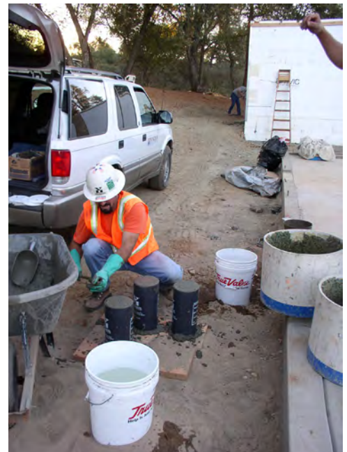
Figure 12 – Taking random samples of concrete for compressive strength testing at 28 days
