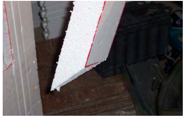
Figure 44 – Making the end cuttings flare out
