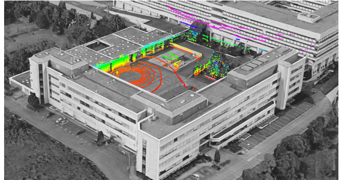
Fig. 1: An exemplary point cloud generated from one scan of the courtyard of the Landesbehördenhaus in Bonn, projected into an aerial photography [4]. Points are colored by height.
