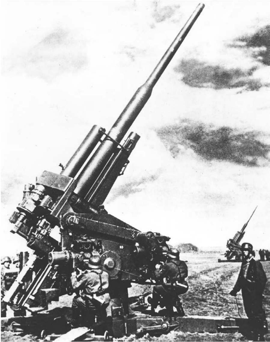
Figure 17. German 128 mm AAA gun. The 128 mm gun was the most powerful anti-aircraft gun the Germans put into service during the war. By the end of 1944, they had deployed about 2,000. (Reprinted from Imperial War Museum.)
