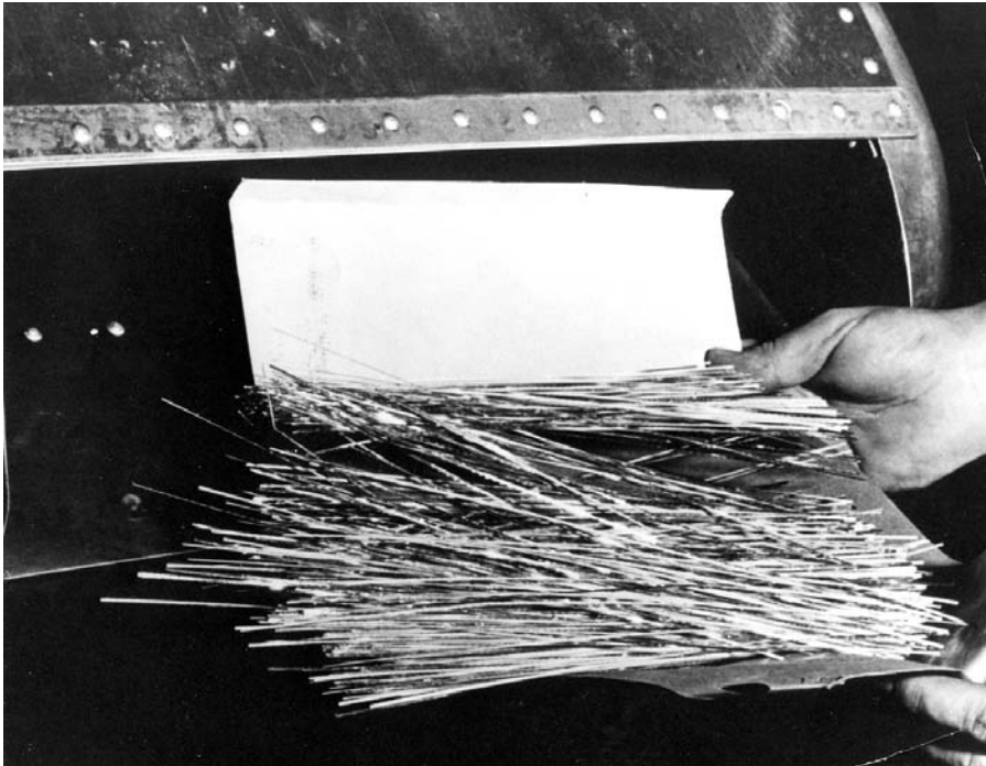
Figure 28. Chaff. Chaff was an effective counter used against radar beginning in World War II. (Adapted from US Army Air Defense Museum.)
