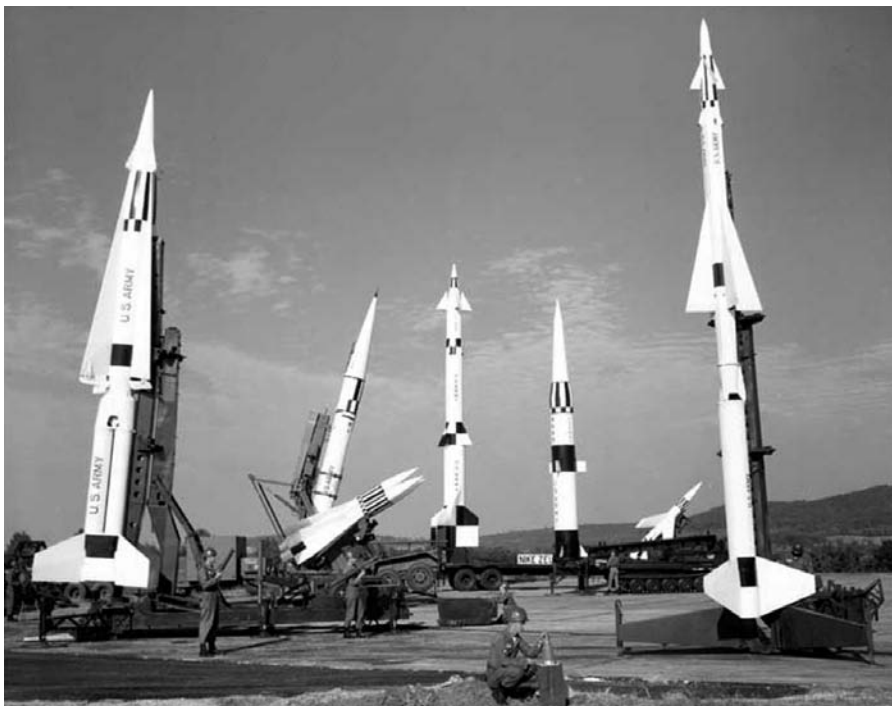
Figure 40. Army SAMs. The US Army fielded an impressive number of both surface-to-air missiles and surface-to-surface missiles. From left to right: Hercules (SAM), (front) Hawk (SAM), (rear) Sergeant, Zeus (SAM), Pershing, LaCross, and Ajax (SAM). The soldiers from left to right are holding LAW, Redeye (SAM), and Entac. (Adapted from Redstone Arsenal.)
