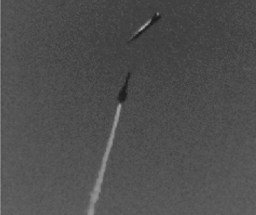
Figure 95. Hawk intercepting Lance. The Hawk had the potential to intercept ballistic missiles, as it demonstrated in intercepting this Lance surface-to-surface missile. (Reprinted from Ballistic Missile Defense Organization.)
