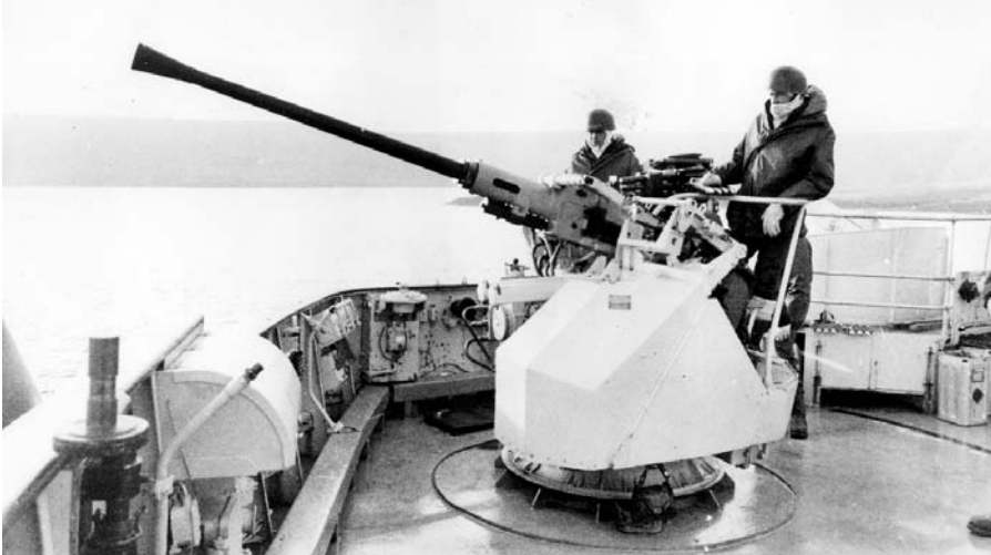
Figure 73. Bofors 40 mm shipboard. In addition to numerous SAMs, the Royal Navy retained guns to protect against air strikes. This Bofors 40 mm L/60 and crew are aboard either the HMS Fearless or HMS Intrepid during the Falklands War. (Reprinted from Imperial War Museum.)
