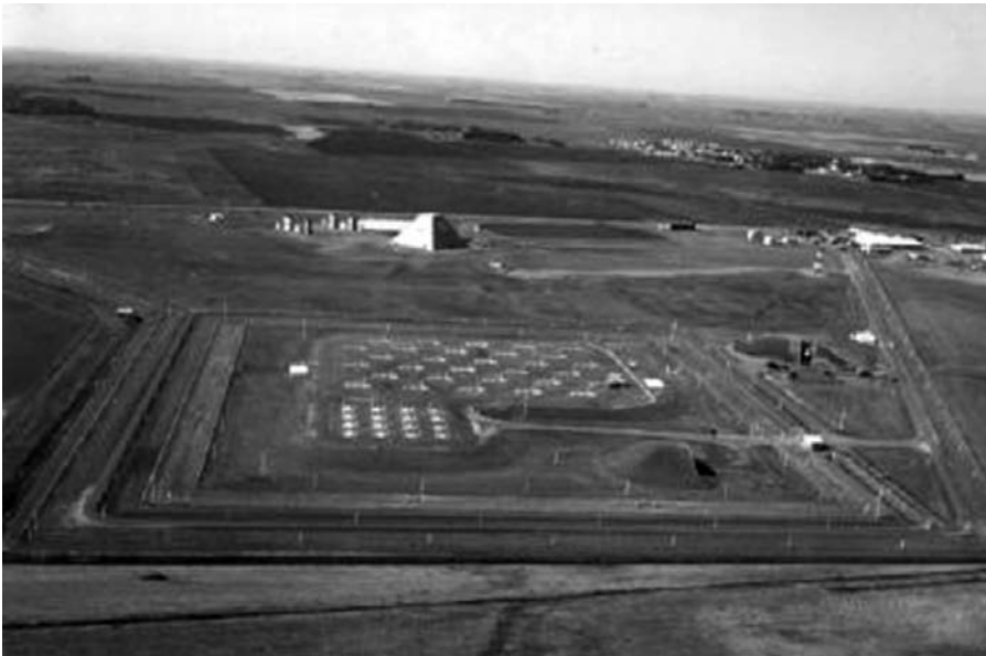
Figure 85. US ABM site at Grand Forks, North Dakota. The 16 round objects in the foreground are Sprint silos, the longish objects behind them are the Spartan silos, and the pyramid-shaped structure to the rear is the missile site radar. (Reprinted from http://www.paineless.id.au/misssile/Hsafeguard.html .)
