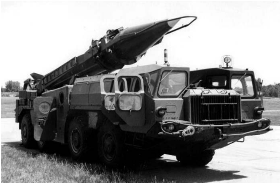
Figure 87. Scud missile. The Iraqis modified the Soviet Scud missile which extended its range but lessened its accuracy. Iraqi Scud attacks put political pressure on the coalition and, as a result, diverted resources. (Reprinted from http://www.acq.osd.mil .)
