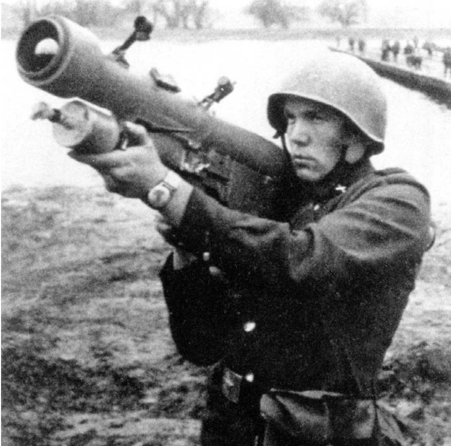
Figure 54. SA-7 Grail. The Soviets quickly developed and fielded man-portable SAMs. The North Vietnamese first used the SA-7 in 1972, and it proved especially effective against slow-moving and low-flying aircraft. (Reprinted from USAF.)
