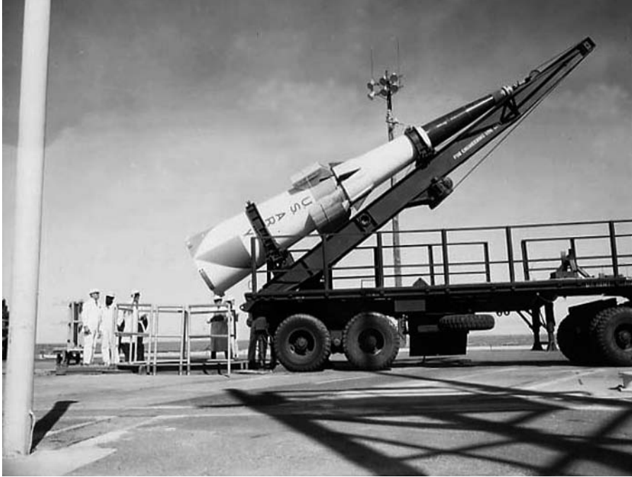
Figure 82. Sprint. The Sprint missile was the short-range component of the American ABM system. It was a high-acceleration missile designed to destroy incoming warheads that eluded the Spartan. (Reprinted from http://www.brook.edu/FP/projects/nucwcost/sprint.htm .)
