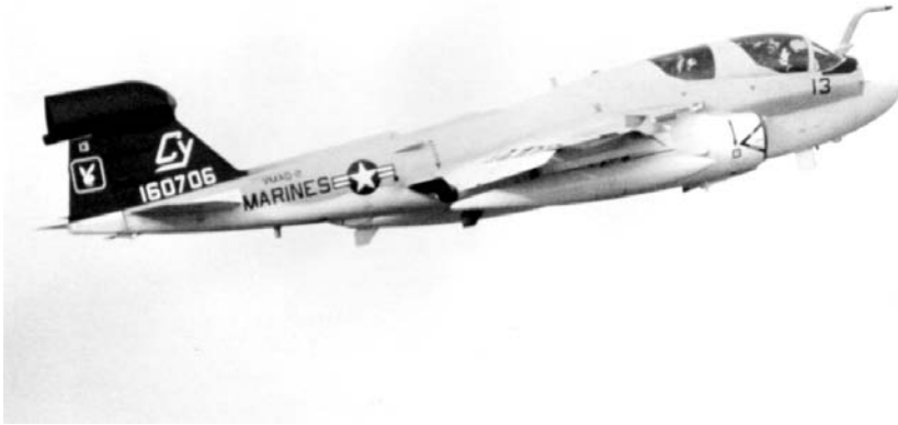
Figure 63. EA-6B Prowler. The EA-6B Prowler carried a four-man crew to jam enemy radars. (Reprinted from USAF.)
