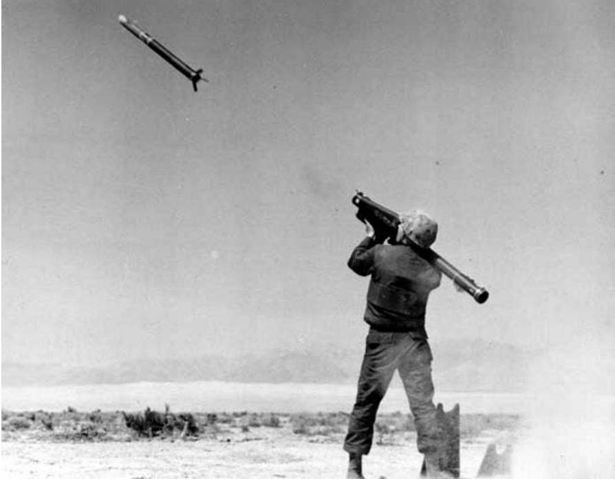
Figure 50. Redeye launch. The Redeye gave the individual American soldier a weapon that could down aircraft. This first-generation missile was limited by its inability to identify friend from foe and restricted engagement envelope. (Reprinted from Redstone Arsenal.)
