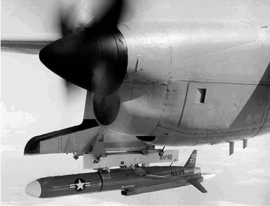
Figure 93. BQM-74 drone. The Airmen used the BQM-74 drone to deceive enemy radars as well as force them to reveal their positions to more active defensive measures. (Reprinted from http://www.multipull.com/twascasefile/bqm74e.gif .)
