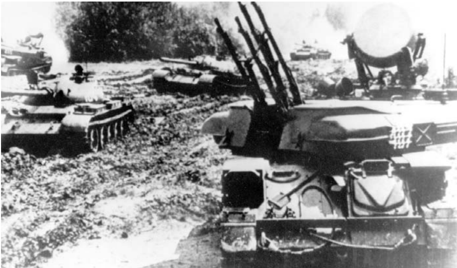
Figure 68. ZSU-23. The ZSU-23-4 proved an unpleasant surprise for Israeli aircraft in the 1973 Middle East War. It mounted four 23 mm cannons guided by radar on a tracked vehicle. (Reprinted from US Army Air Defense Museum.)
