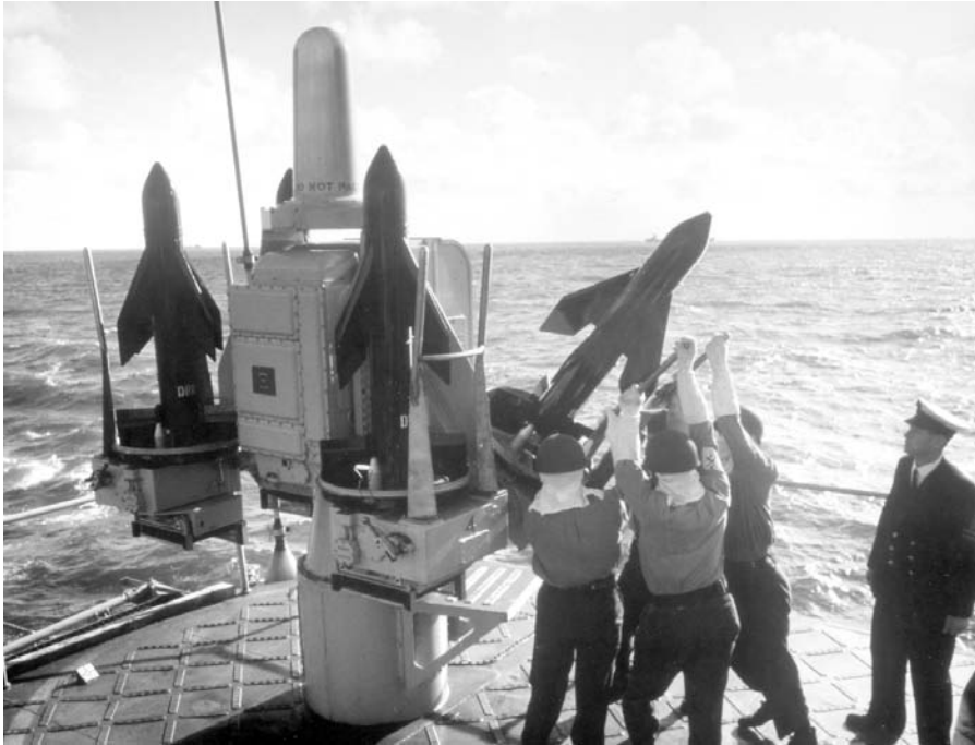
Figure 76. Seacat. The short-range British Seacat was an older SAM used by the Royal Navy, as well as by the Argentines. There is some dispute as to its effectiveness in the Falklands War. This picture is of a training exercise before that war. (Reprinted from Imperial War Museum.)
