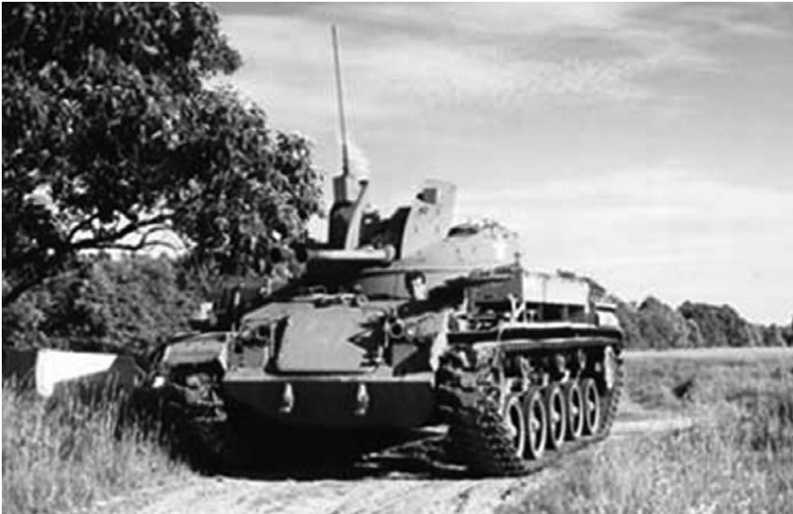
Figure 35. Duster. The Duster was one of a number of failed Army anti-aircraft projects. It mounted two 40 mm guns on a tracked vehicle. (Reprinted from http://www.militaryhistorymuseum.org/gallery.html .)
