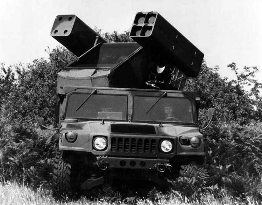
Figure 52. Avenger. The Avenger consisted of a turret with Stinger missiles mounted on the ubiquitous Hummer. (Reprinted from Redstone Arsenal.)
