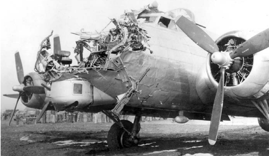
Figure 27. Damaged B-17. This B-17 survived a flak hit over Cologne, Germany. During World War II, the Eighth Air Force suffered 20 percent damage per sortie and wrote off 1,600 bombers as “damaged beyond economic repair.” (Reprinted from USAF.)
