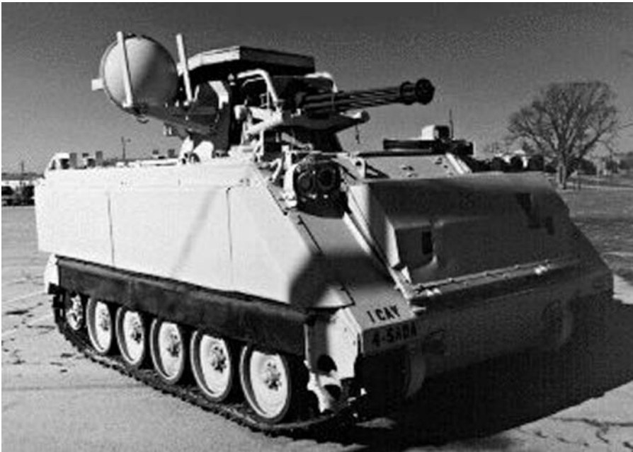
Figure 38. Vulcan M163. The Army mounted the 20 mm Vulcan gun with radar guidance on an M163 armored personnel carrier. (Reprinted from http://www.relli.com/weapons.htm .)
