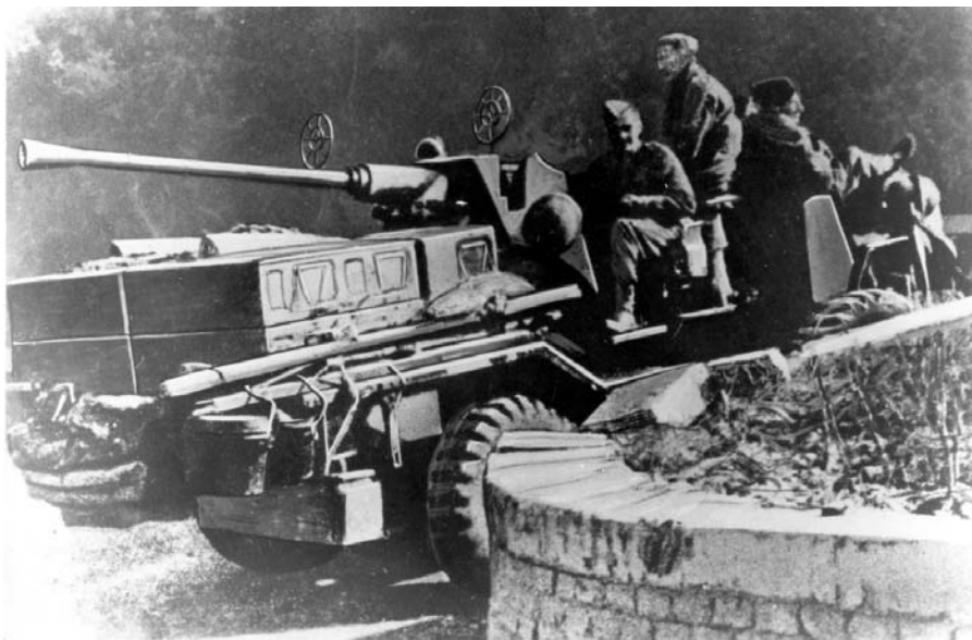
Figure 15: German 40 mm Bofors. The Germans used a wide variety of light flak guns including this truck-mounted 40 mm Bofors. (Adapted from Air Force Historical Research Agency.)
