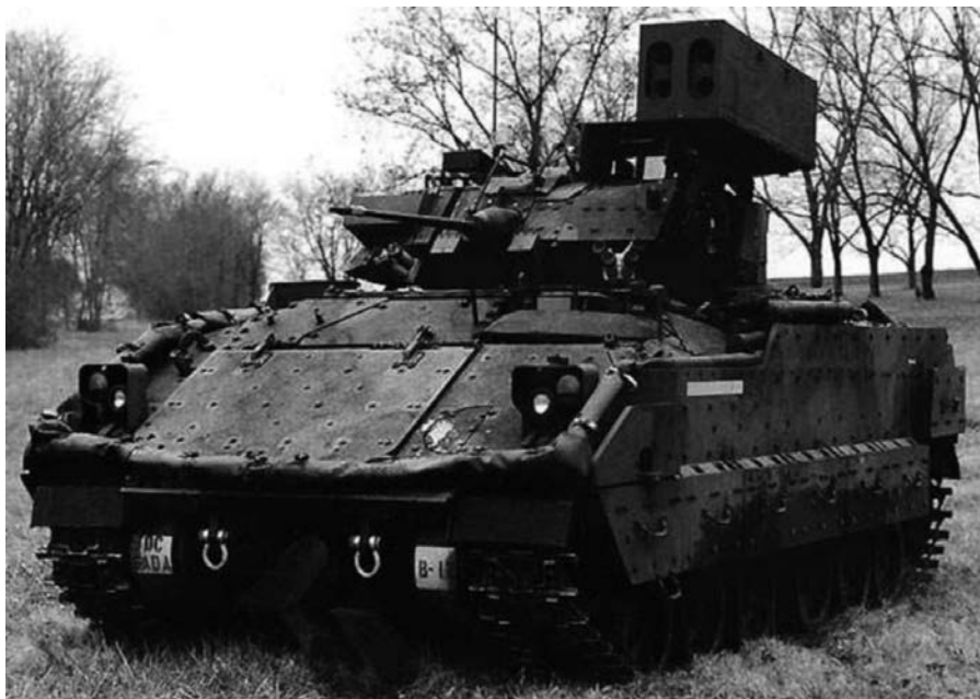
Figure 53. Bradley Linebacker. The Bradley Linebacker mounted four Stinger missiles atop a Bradley fighting vehicle. (Reprinted from internet: army-technology.com.projects/linebacker1.htm .)
