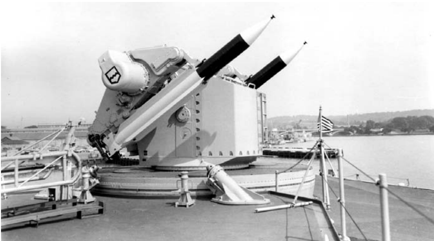
Figure 65. Terrier. A Terrier downed a MiG in 1972, one of three MiGs destroyed by Navy SAMs. This Terrier is mounted on the USS McCormick . (Reprinted from USAF.)
