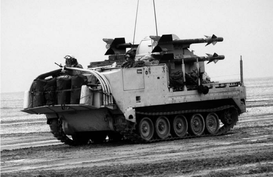
Figure 49. Chaparral. The Chaparral consisted of a Sidewinder air-to-air missile adapted for surface-to-air operations. Intended as an interim, short-term measure, it saw much longer service, including—as seen here—in the first Gulf War. (Adapted from Defense Visual Information Center.)
