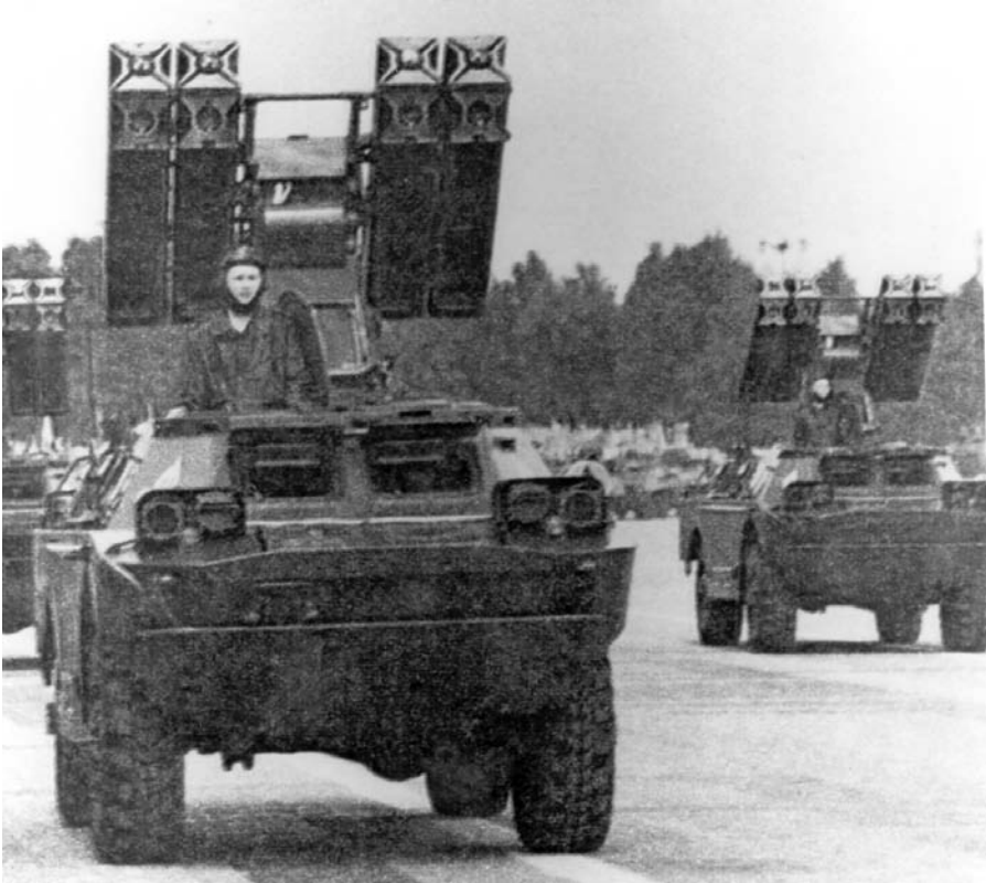
Figure 69. SA-9. The Soviet SA-9 mounts eight SA-7 missiles on a mobile platform. (Reprinted from USAF.)
