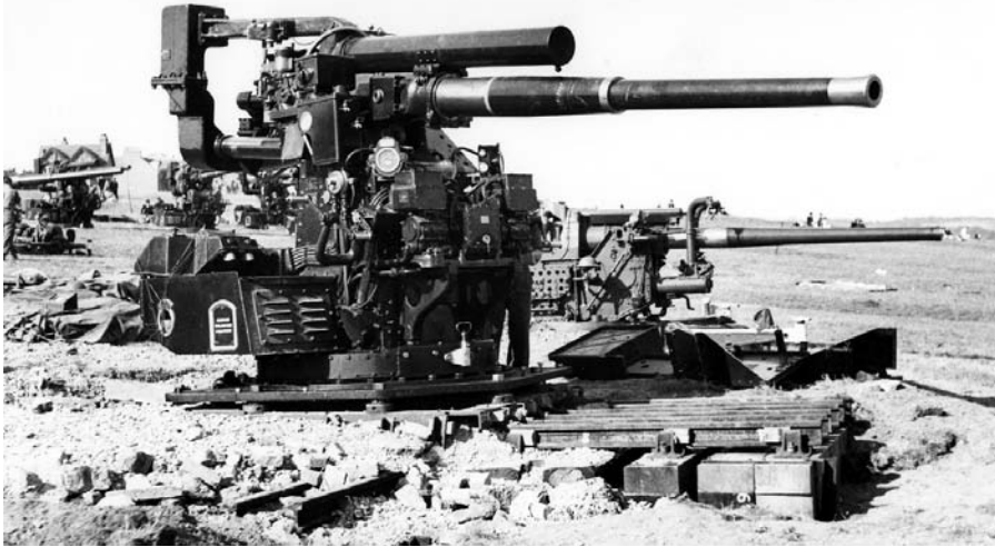
Figure 4. 3.7-inch gun on a Pile mattress. Here it is mounted on a “Pile mattress” used during the V-1 campaign and named for anti-aircraft artillery commander Gen Frederick Pile. (Reprinted from Imperial War Museum.)
