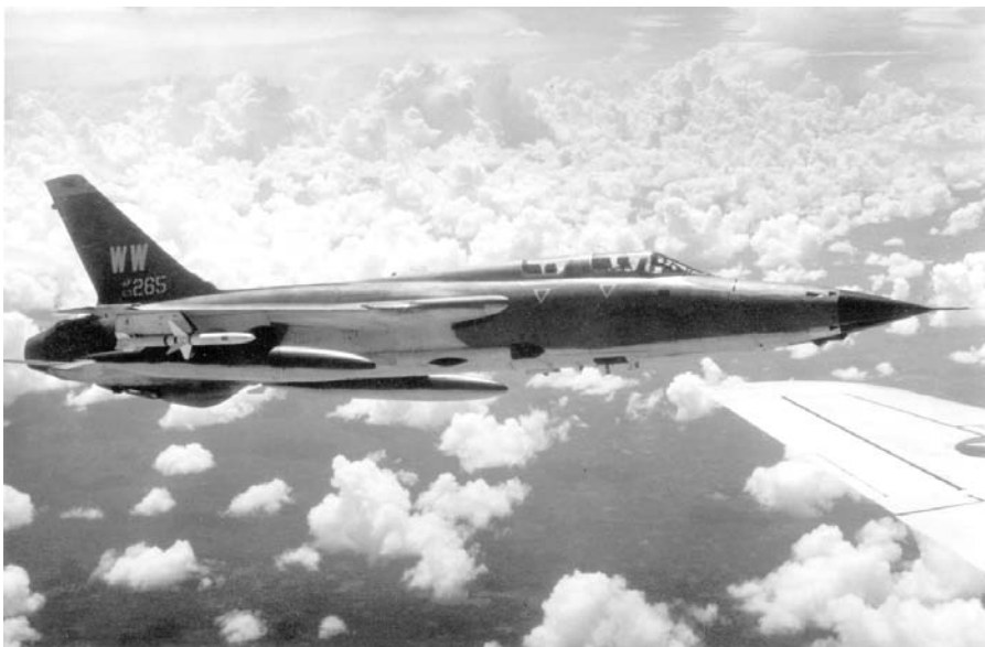
Figure 61. Wild Weasel. The USAF employed special units, called Wild Weasel, to attack Communist radar. This two-seat F-105G is carrying two Shrike antiradiation missiles. (Reprinted from USAF.)
