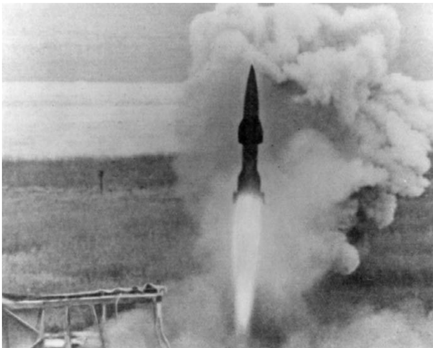
Figure 25. Wasserfall. Wasserfall at Peenemünde in the fall of 1944. It was a smaller version of the V-2 and the largest of the German flak rockets. (Adapted from Air Force Historical Research Agency.)
