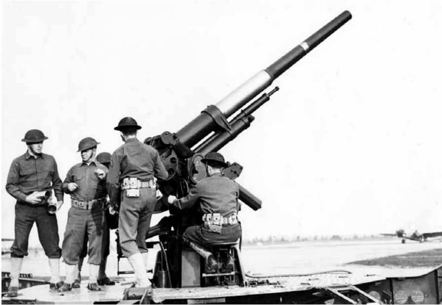
Figure 2. Standard US heavy AAA gun during the interwar years. The standard US heavy AAA piece during the interwar years was this three-inch gun. Members of the 62d Coast Artillery engage in a practice exercise in August 1941. (Reprinted from USAF.)
