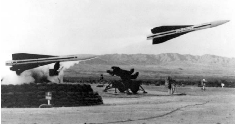
Figure 46. Hawk launch. The Hawk went into service (1959) only a year after the Nike Hercules. Whereas the Nike family was only employed from fixed installations, the Hawk was mobile. (Reprinted from US Army Air Defense Museum.)
