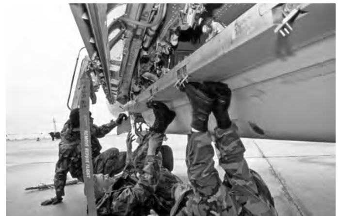
These 366th TFW maintainers were not exercising to improve their PT grades, but were trying to close the doors of the canoe-shaped radome manually. It was mounted under the fuselage, occupying the old bomb bay space and housed the antennas for the high-powered jamming transmitters. (Guy Aceto)
