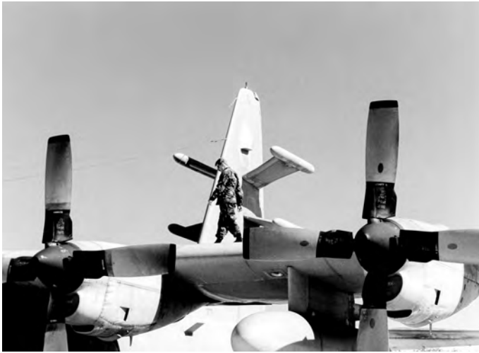
A maintenance technician is performing a pre-mission check while on the wing of one of the four RIVET RIDER EC-130Es. The four fin-mounted pods contain the TV antennas. The aircraft were later modified with, among others, enhancement of self-protection (IR jammer and chaff/flares) and addition of WWCTV (Worldwide Color Television) capability. Modifications were performed during PDM at Lockheed Aircraft Services in Ontario, Calif. (LMAS, John Rossino)
