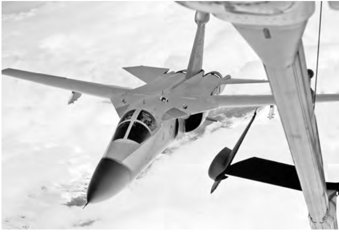
An EF-111A Raven about to be refueled by a KC-10A Extender. (USAF, SSgt Kevin Bishop)
