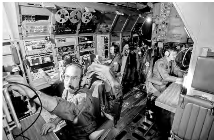
The broadcast studio in the cargo hold of the EC-130E VOLANT SOLO with six crew members and their (off-the-shelf) equipment. TSgt Barry Hein, foreground, an electronic communication systems operator, is coordinating a broadcast mission. (USAF, TSgt John McDowell)
