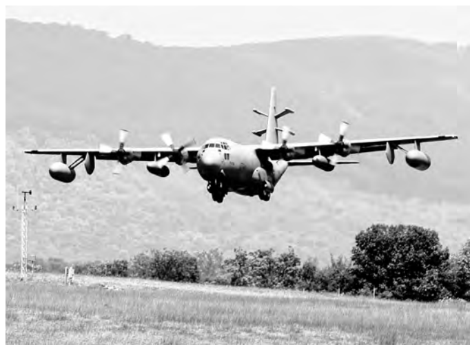
EC-130E 63-7773 on finals on March 28, 2006. Together with 63-7869 it arrived at KFIA on August 31, 1990. It flew its final sortie from King Fahd on February 25, 1991 for a total of 577.3 flying hours, was replaced there by 869 and deployed to Incirlik to support Operation PROVEN FORCE. The bulky pods on the outboards contain the WWCTV (Worldwide Color Television) VHF/UHF TV broadcasting equipment. 773 is on display at Fort Indiantown Gap, home of the Pennsylvania National Guard. (USAF, SSgt Matt Schwartz)
