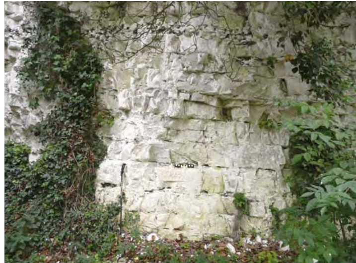
4. Detail of lower face to left of cleared section in photo 2, showing prominent layer of irregular flints near top (probably the Cote Bottom Flint) and thinner flint layers towards the base including a layer of tabular flints. 1m pole for scale. Grid ref. TQ11540638. Direction SE.
