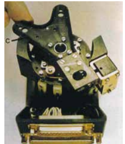
Fig. 1. Example of a scanning mechanism from an Earth observation satellite. The Y-shaped so-called anchor is made to oscillate from its 'middle' resting position by electromagnetic forces. In doing so, the anchor continually impacts and is rebounded from each of the end stops. Eventually this anchor became cold welded to the end-stop, labelled C in the photograph.
