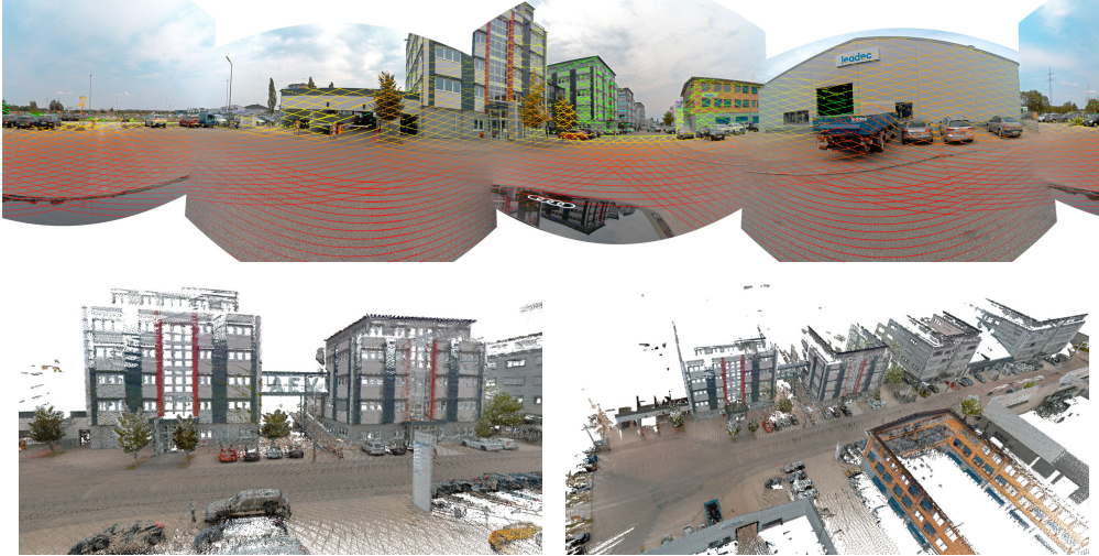
Figure 3: Upper panel: Mapping of LiDAR points onto stitched camera images. Lower panels: colored 3D maps generated from a 30 second sequence using an ICP-based open-loop SLAM.
