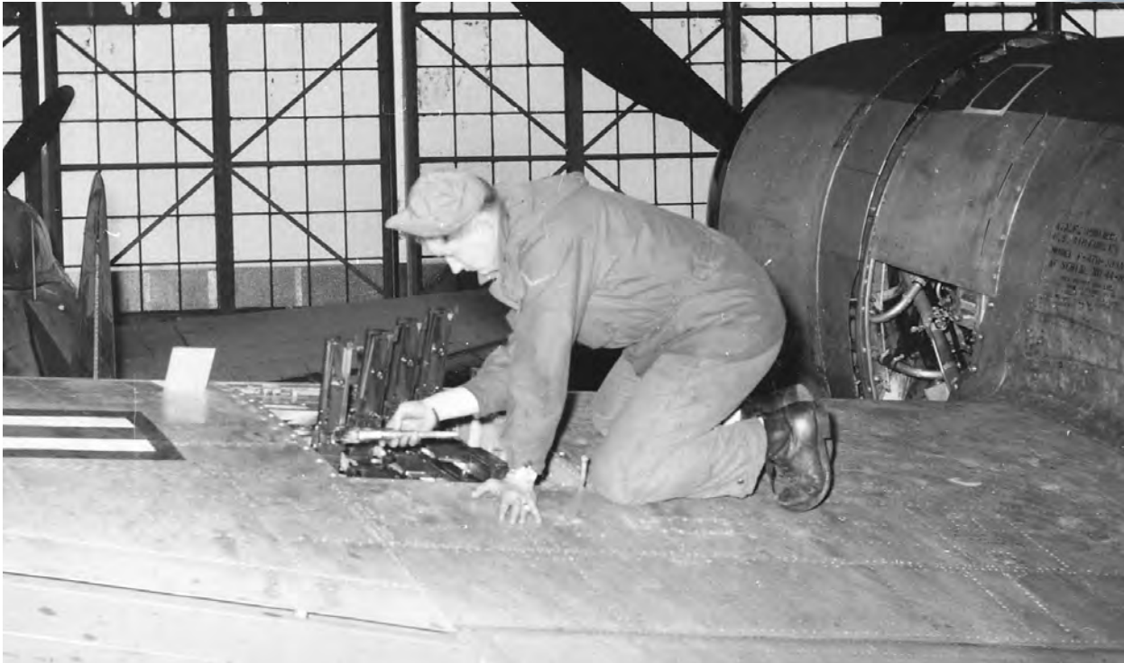
Working on the P-47 aircraft machine guns. (Courtesy Elzear G. "Al" Houle)
