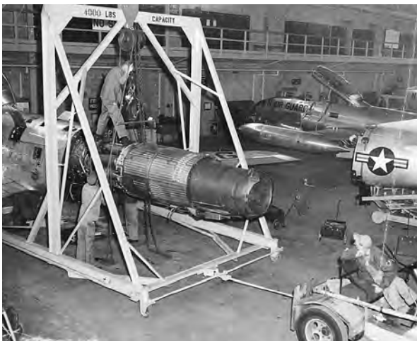
Red Tail Flight: CMSgt. Bill Lefebvre watches from the tug as the crew installs an F-86L engine, circa 1957. (Courtesy Walter Colby)
