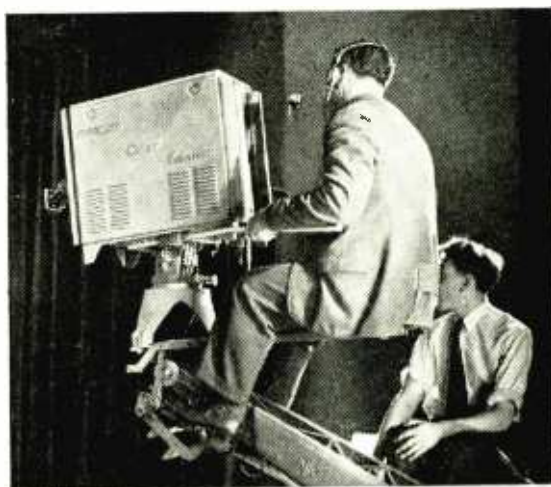
Colour television camera used with the Marconi system referred to in the article. It has only two pick-up tubes (one for high-definition monochrome information and the other for low-definition colour) and is notable for its small size.
