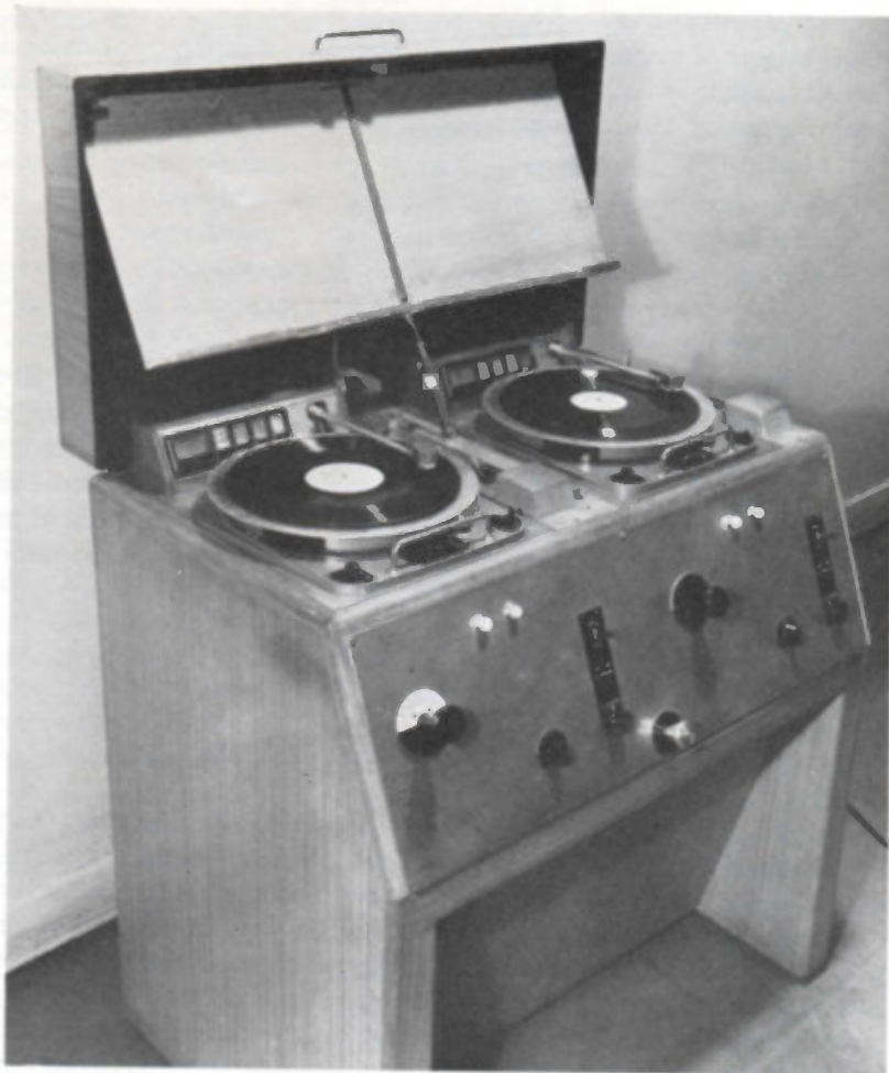
BBC disc reproducing desk, type RP2/1. The equipment can be used at speeds of 33 \frac{1}{3} , 45, and 78 r.p.m. and includes groove-location and quick starting facilities
