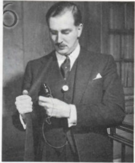
(left) 'Suit-case' outside broadcast equipment (right) BBC Radio Microphone, showing the transmitter being slipped into a pocket. The battery-pack is of similar size, the aerial is concealed in the clothing and the miniature microphone can be replaced by a hand-held type for interviewing
