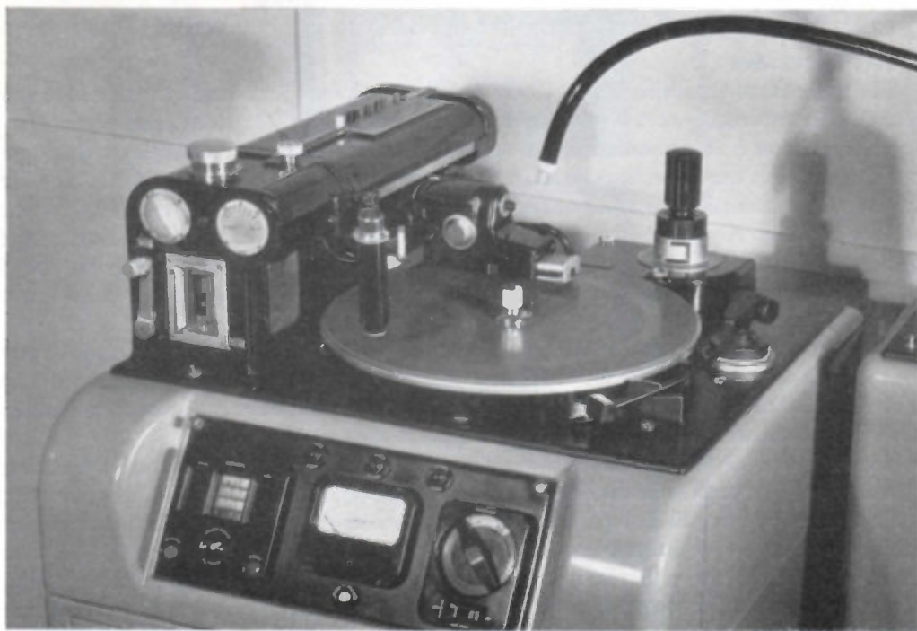
High performance disc recording equipment, type D, designed and produced by the BBC
