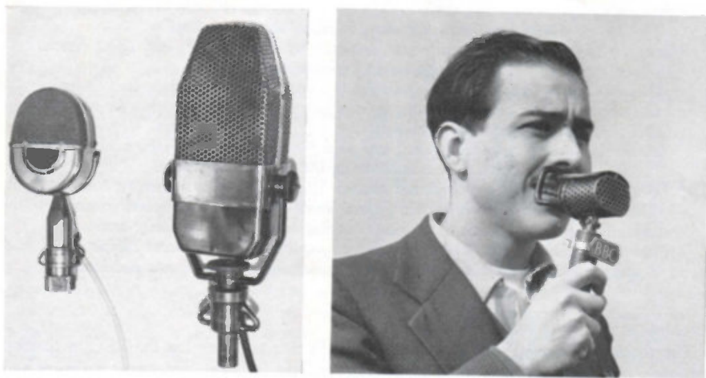
(left) Ribbon microphones—type PGS and AXBT to same scale (right) Noise-cancelling lip microphone, type L2
