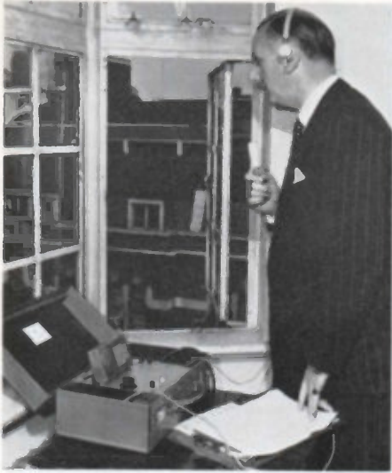
(left) 'Suit-case' outside broadcast equipment (right) BBC Radio Microphone, showing the transmitter being slipped into a pocket. The battery-pack is of similar size, the aerial is concealed in the clothing and the miniature microphone can be replaced by a hand-held type for interviewing
