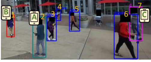
(a) An example screenshot from the experiment. 7 pedestrians are detected by human detector. 3 pedestrians' phones are exchanging FTM messages with the WiFi access point while recording IMU measurements.
