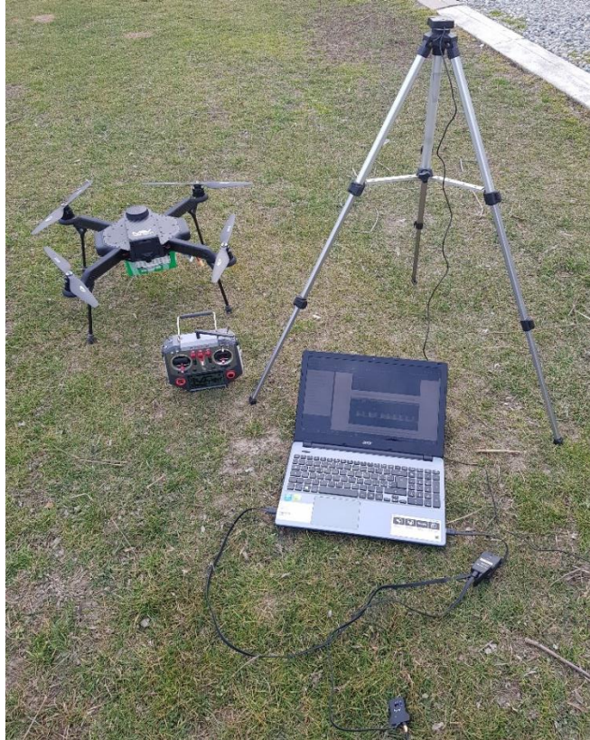
Figure 71: Base and rover configuration – integration onboard a Mavtech UAV
