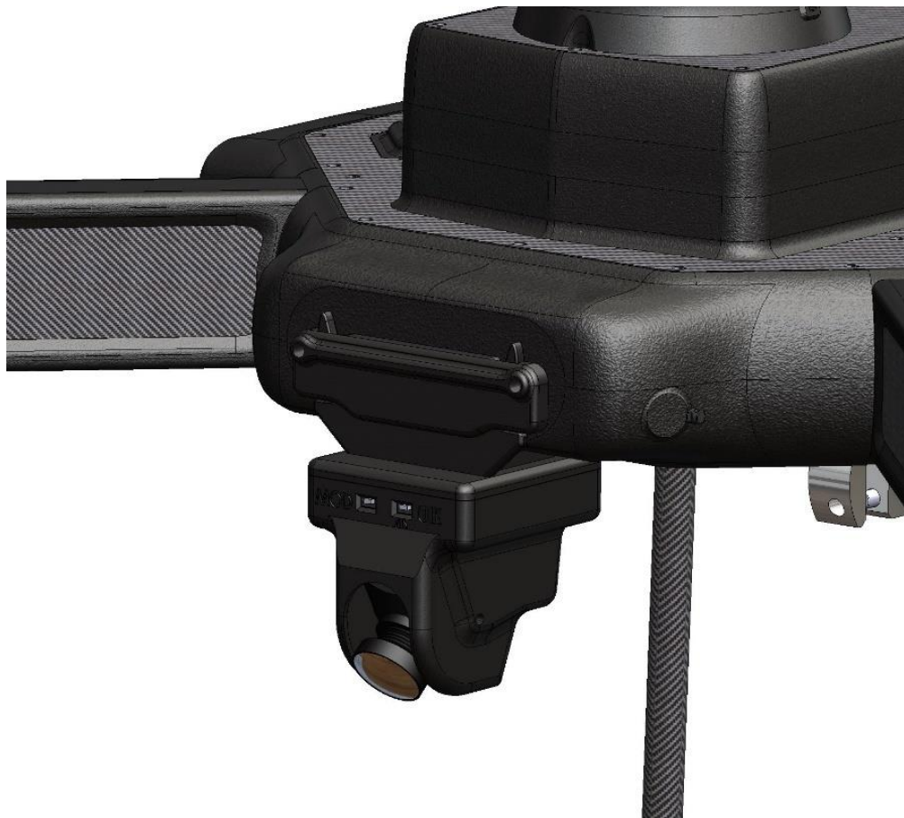
Figure 18: Navigation camera - CAD integration system
