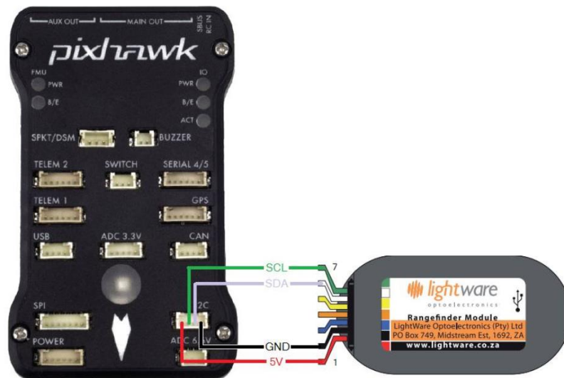
Figure 16: I2C interface connections between altimeter and autopilot
