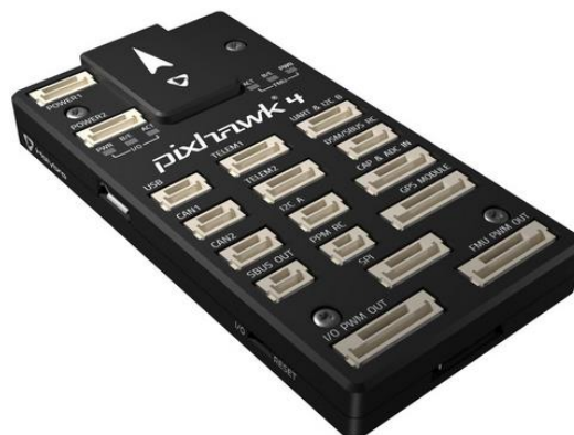
Figure 11: Holybro Pixhawk 4 autopilot (48)
