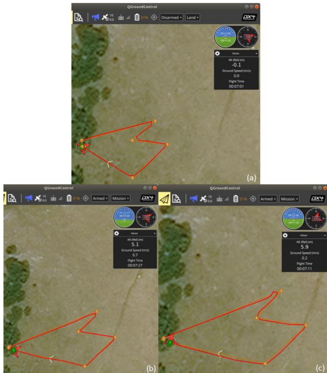
Figure 61: No obstacle simulations – reaching waypoints with greater accuracy
