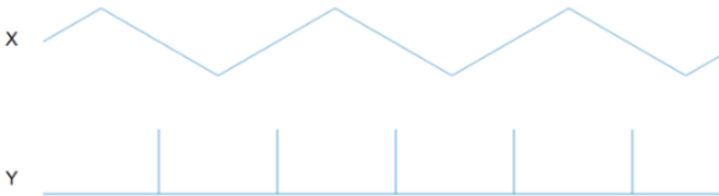
Figure 8: Tennis Court Waveforms. Waveforms required to produce the static tennis court for our game
