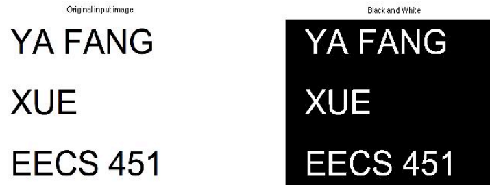
Fig.1 Original input image and after binarization
