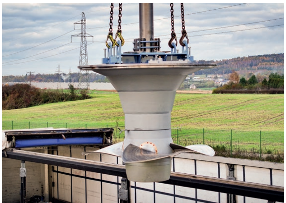
Fig. 2. Transport of the turbine runner
