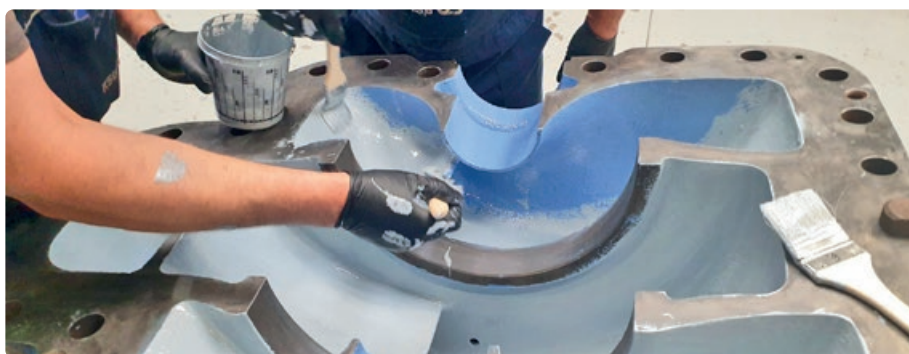
Photo 6. BELZONA(1341) composite coating in a rotodynamic pump
