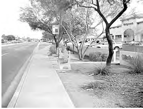
Figure 2.9.4.2.a: A sidewalk with no landscape buffer feels like it is a part of the roadway.
