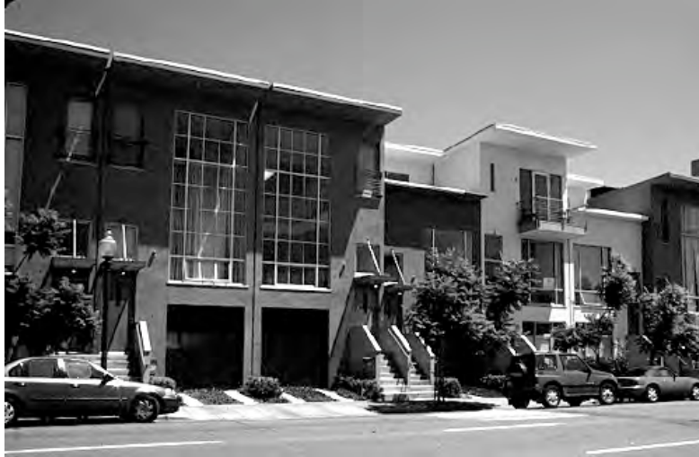
Figure 4.3.2: Front stoops and stairs raise the living area well above the street creating privacy for residents. Although garages front onto the sidewalk, they do not dominate and are well detailed.
