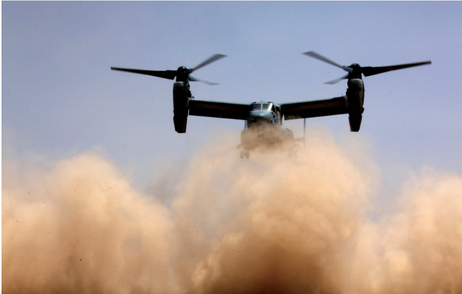
An MV-22B with VMM-365 lands in “brown out” conditions in Helmand Province, Afghanistan in July 2010. Dust and sand take their toll on engines, sometimes needing replacement after “just a few hundred hours.” (US Marine Corps)
