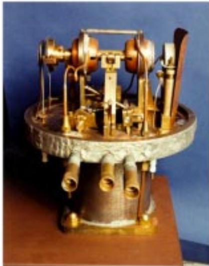
**Fig 7.** The Varian Two-Cavity Klystron
