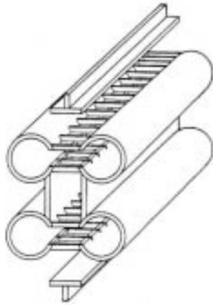
**Fig. 12** Kovalenko's Sheet-Beam Klystron
