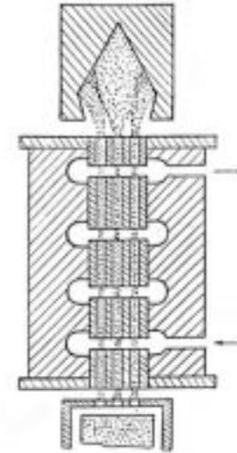
**Fig. 13** Sketch of Russian Multiple Beam Klystron
