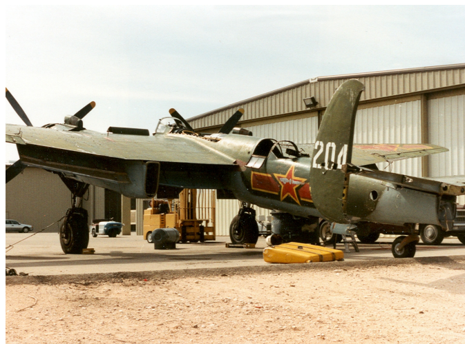
▲ This undated photo shows the Museum's Tupolev Tu-2, still with Chinese Air Force paint and markings, being reassembled on the ramp in front of the maintenance hangar.
