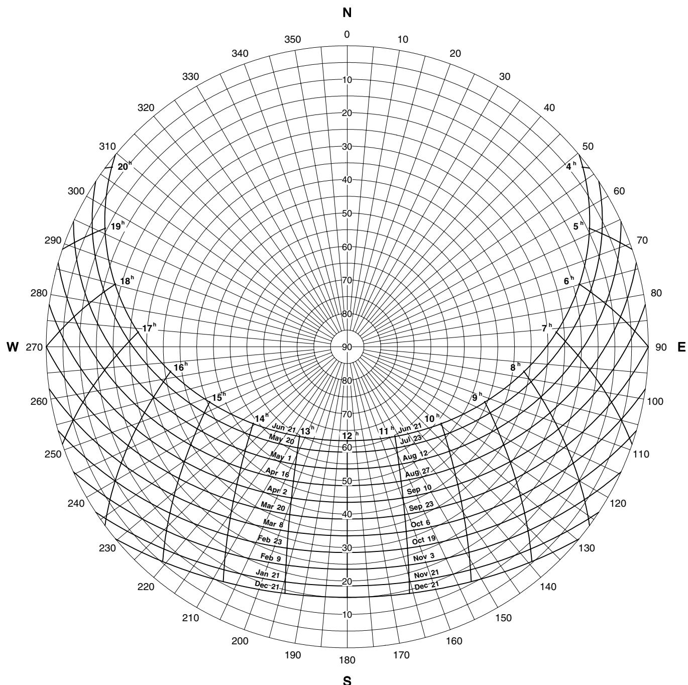
The diagram shows the altitude and azimuth of the Sun for a range of local apparent solar times from sunrise to sunset at latitude N 51° 30' (which is the latitude of London) for a series of dates throughout the year. A separate diagram for a specific latitude, which may be needed for better accuracy, will be supplied upon request.
