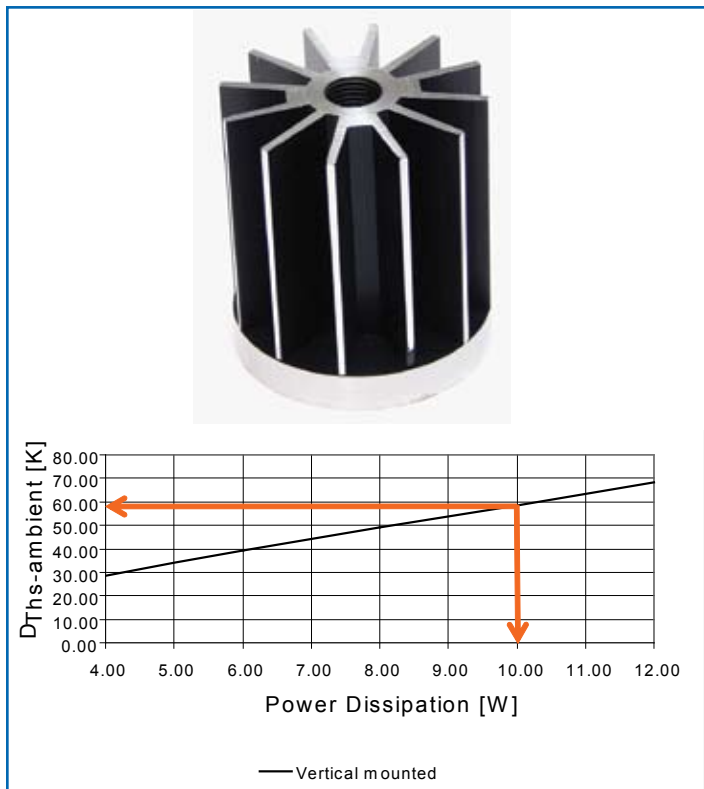
Figure 6. Experimental Results using the ATSEU-077B-C4-R0 Heat Sink.
