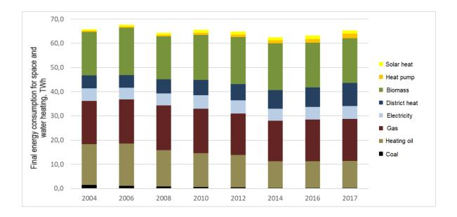
Figure 3 Energy consumption from all sources for space and water heating in all households Source (Statistics Austria, 2019)
