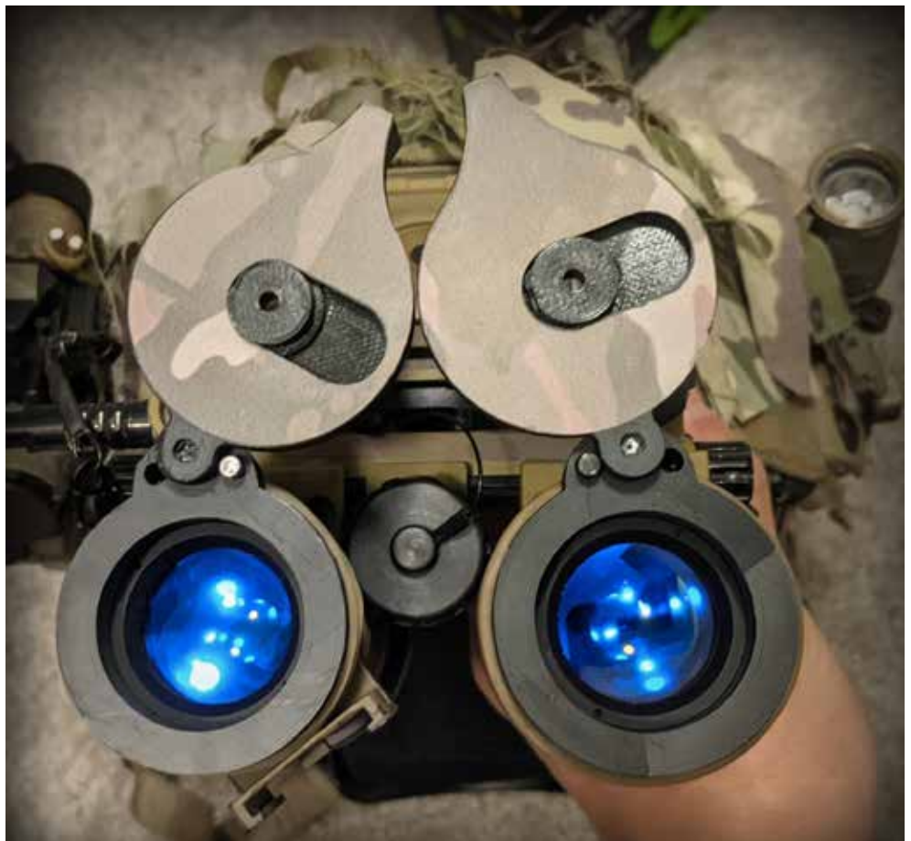
Dark Focus Concepts FRS increases DOF. It swivels up, as pictured, for more light gathering.
