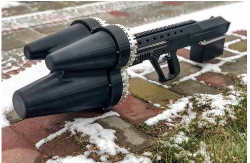
The "Riff" is a man-portable, battery powered anti-drone weapon manufactured by InterProInvest and built on a polymer chassis using Malyuk rifle parts.
