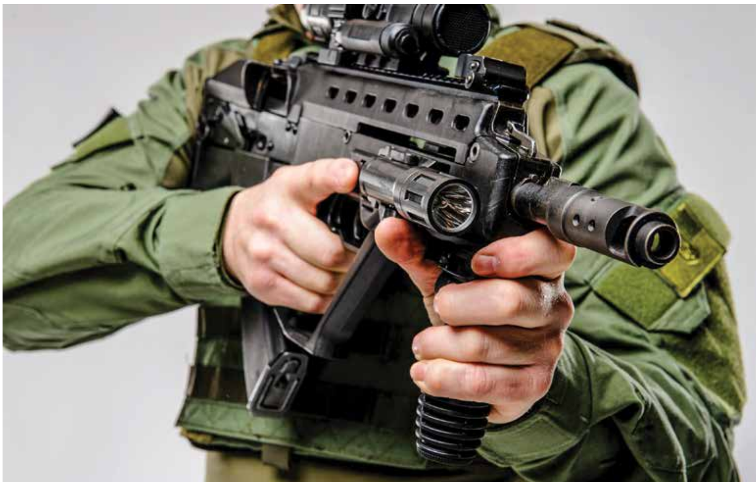
The lever located just over the barrel, clearly visible in this photo, is not a gas regulator but a retaining latch that must be fully rotated counterclockwise to allow field stripping.
