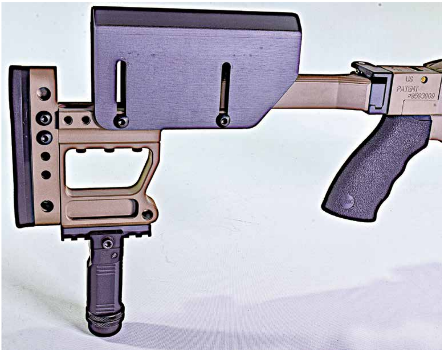
The G10's foldable stock is also adjustable for length of pull, comb height and recoil pad position.
