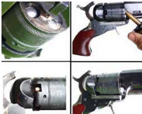
Loading sequence for percussion revolvers.
