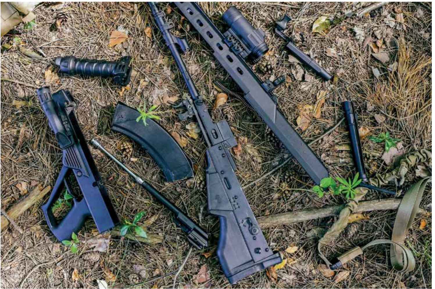
The field strip reveals the high commonality of components between the Malyuk and the legacy, conventional AKM and AK-74M rifles.
