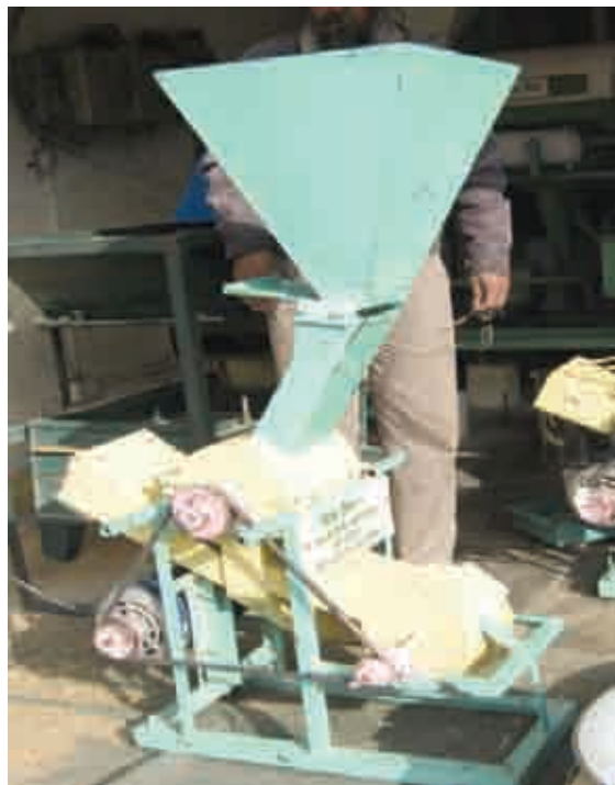
Vivek Thresher-cum-Pearler for Finger millet and Barnyard millet was developed by Vivekananda Parvatiya Krishi Anusandhan Sansthan (ICAR), Almora (Uttarakhand).
