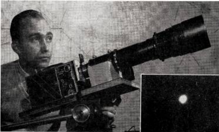
USING a camera equipped with a 40-in. telephoto lens, Skip Nelson, assistant photo director at KSTP-TV St. Paul-Minneapolis (above), caught Sputnik II as it streaked across the sky just east of Minnesota Nov. 5. A prismatic rifle spotting telescope was placed beside the camera for use as a viewfinder. Result: clear 16 mm motion pictures of the satellite (inset) which were sent to Chicago and used on an NBC news show the next day.
