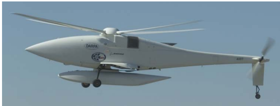
Figure 20: A160 long endurance unmanned rotorcraft demonstrating a 1000 pound payload carriage capability over a distance of 962 kilometers during an eight hour flight in September 2007.
