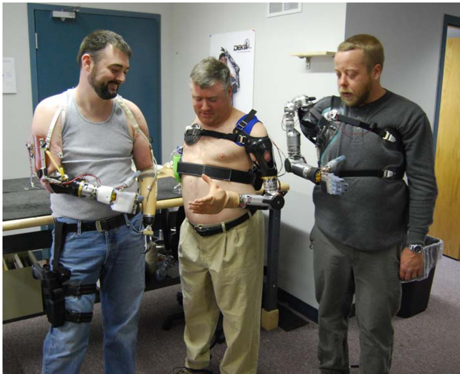
Figure 34: DARPA’s revolutionary non-invasively controlled advanced prosthetic, developed under the Revolutionizing Prosthetics 2007 program.
