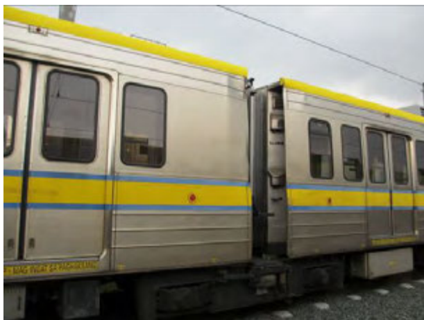
Figure 5.1-2 2G Rolling Stock: Body is deformed by collision (1107)
