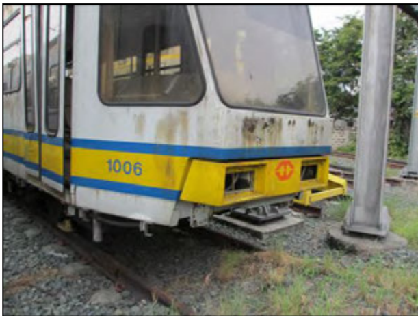
Headlight and bumper are missing (1006)
