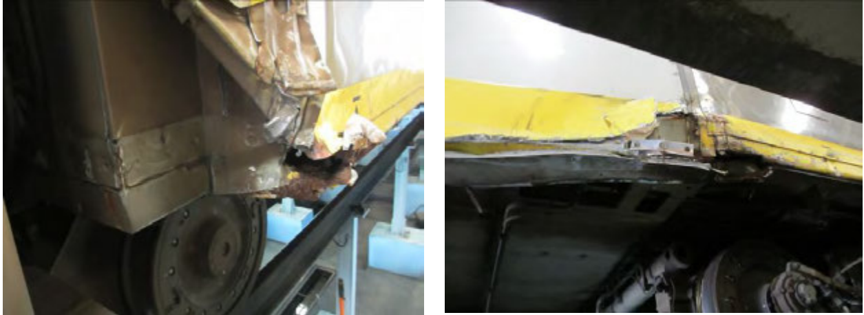
Figure 5.1-3 3G Train: Body shell is turned outward (1236)
