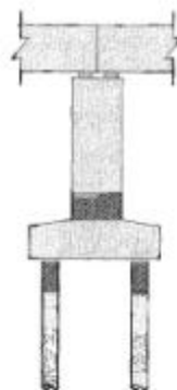
■: Potential damage region
