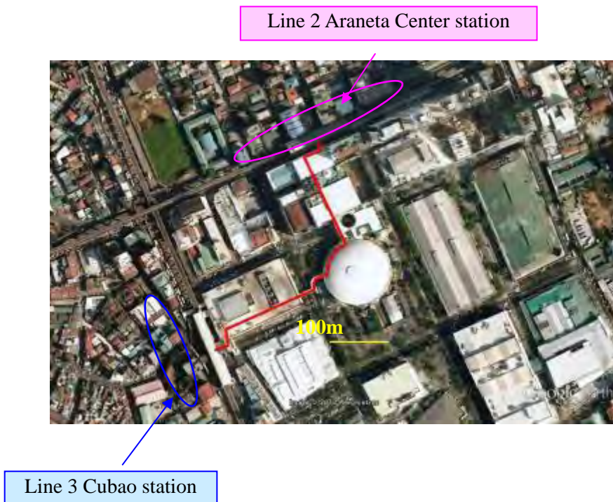
Figure 12.3-2 Interconnection with Line 2 and Line 3
