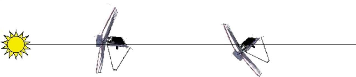
Figure 4. Definition of Sun pitch and Sun roll angles [7]. The S_1 , S_2 and S_3 axes are respectively parallel to the J_1 , J_2 and J_3 axes, with a different origin.
