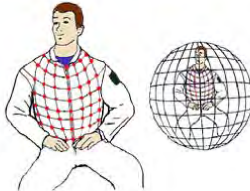
Tactile Situation Awareness System
