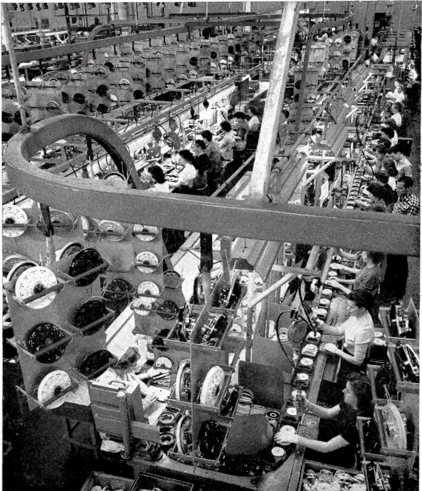
MANUFACTURING Bell telephones is the major function of Western Electric's plant in Indianapolis. The girls above are working on the final assembly of telephone dials. Western Electric also has major manufacturing locations in 12 other cities where we make cable, wire, switchboards, relays, and many other different kinds of telephone equipment and apparatus for the Bell Telephone System, as well as defense products for the Government.
