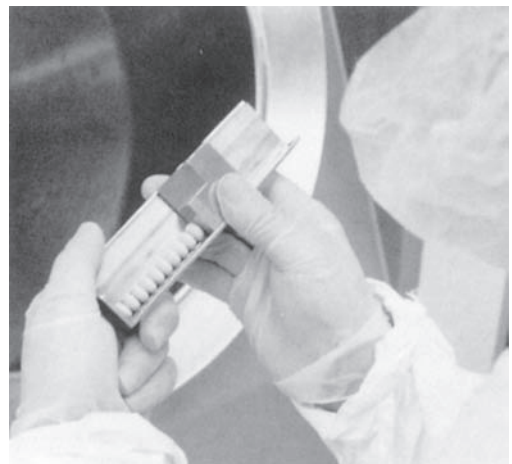
FIGURE 8.32 Gauge used to measure coated tablets. (Courtesy of Eli Lilly and Company.)
