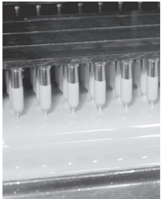
FIGURE 7.3 Capsules being dipped for coloring on automated capsule-making equipment. (Courtesy of Shinogi Qualicaps.)
