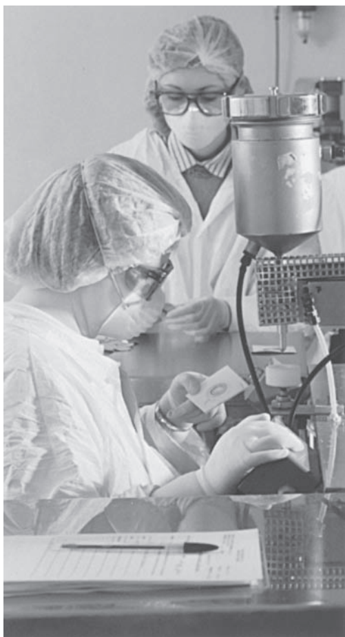
FIGURE 11.8 Pilot-scale manufacture of transdermal patches. (Courtesy of Elan Corporation, plc.)
