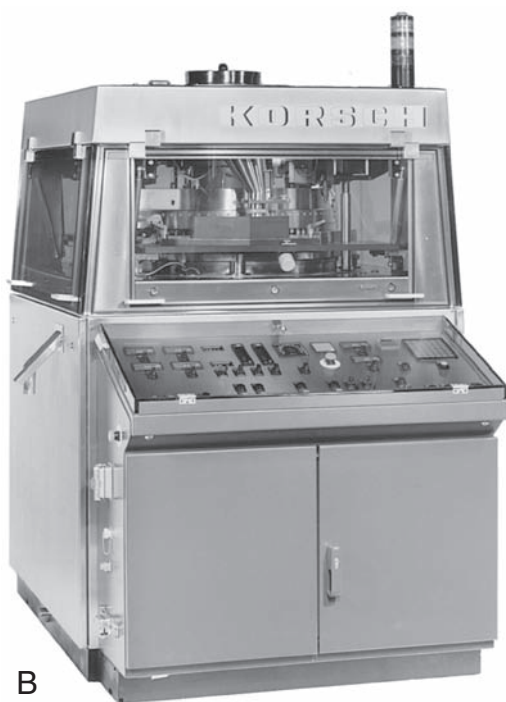
FIGURE 8.1 A. MiniTABLET Press for development and small scale production (Courtesy of GlobePharma). B. High-performance double rotary tablet press. The Korsch PharmapressR has a maximum output of 1 million tablets per hour, but for continuous operation, it is generally run to produce 600,000 to 800,000 tablets per hour. (Courtesy of Korsch Tableting.)
