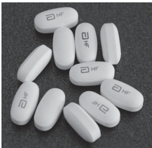
FIGURE 8.34 Coated, polished, and monogrammed tablets. (Courtesy of Wyeth-Ayerst Laboratories.)
