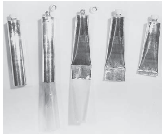
FIGURE 10.7 Steps in the manual filling of ointment tubes.
