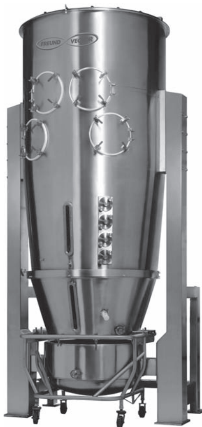
FIGURE 8.35 Vector/Freund Flo-Coater production system. A fluid bed system used to apply coatings to beads, granules, powders, and tablets. Capacity of models ranges from 5 to 700 kg. (Courtesy of Vector Corporation.)
