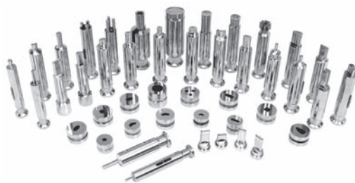
FIGURE 8.2 Various punches and dies for the production of distinctive tablets. (Courtesy of Cemach Machineries Ltd.)
