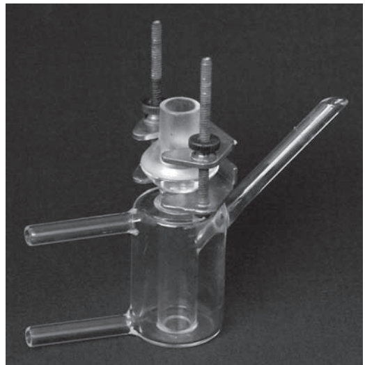
FIGURE 11.2 Typical Franz diffusion cell. The donor cell is on top and the upper and lower chambers are separated by either a membrane or skin. A solution or semisolid containing the drug is placed in the upper cell and a receiver solution in the lower cell. The angle tube on the right is for sampling and fluid replacement. The two ports on the left consist of an inlet and outlet where constant temperature water can be circulated.
