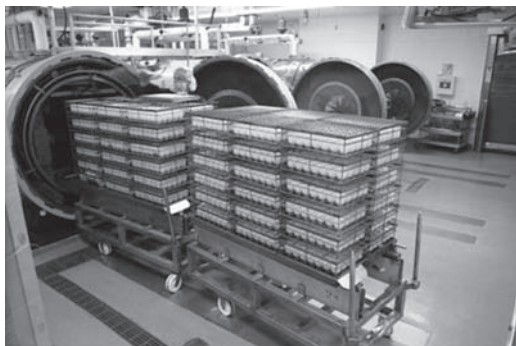
FIGURE 15.3 Autoclaving of intravenous electrolyte solutions. (Courtesy of Hospira, Inc.)
