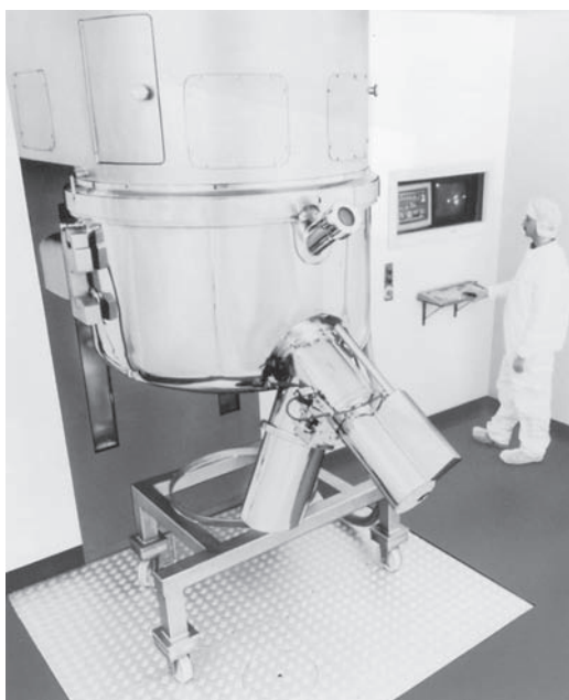
FIGURE 8.22 Microwave vacuum processing in which tablet ingredients are dry-mixed, wetted with a binding liquid, and dried by vacuum and microwave in a single piece of equipment. (Courtesy of GEL Processing.)
