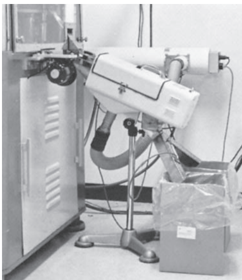
FIGURE 8.28 Model 25 Manesty Tablet Deduster. Tablets leaving the tableting machine are dedusted and passed into the collection containers. (Courtesy of Eli Lilly and Company.)
