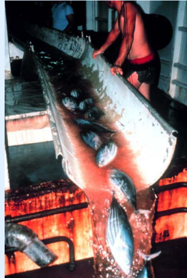
4 The chute leads directly to the freezer compartments
