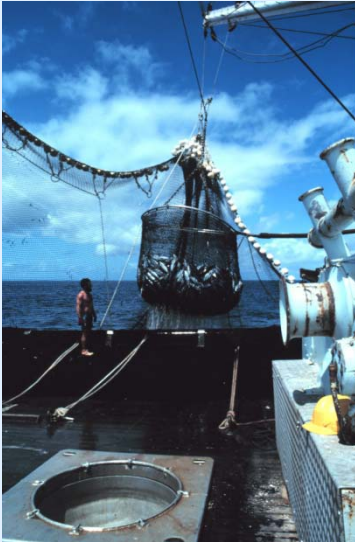
2 The brail net is then placed directly over the hole in the foreground
