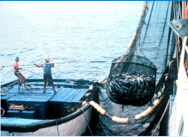
1 The brail net is dipped repeatedly in the seine net, lifting out the fish
