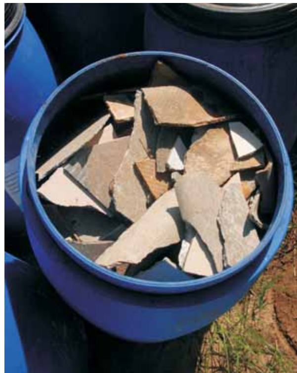
Local teams were trained on the clearing and storage of hazardous waste, including asbestos containing materials, as pictured below.
