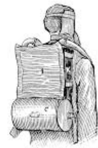
Fig. 35 I. Breathing bag. C. Oxygen cylinder. K. CO 2 absorbent chamber.
