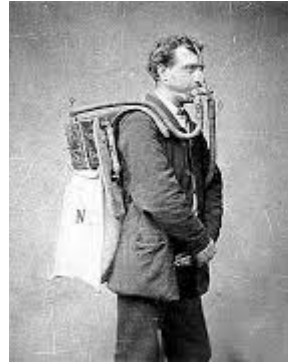
Fig. 35 I. Breathing bag. C. Oxygen cylinder. K. CO 2 absorbent chamber.
