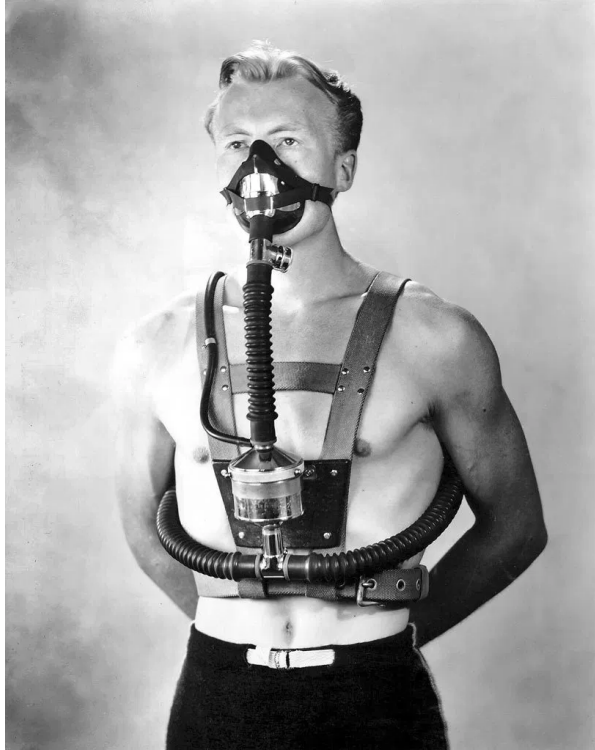
1940: Dr. Christian Lambertsen in the USA designed a 'Self-Contained Underwater Oxygen Breathing Apparatus' for the U.S. military. It was a rebreather. It was the first device to be called SCUBA.
