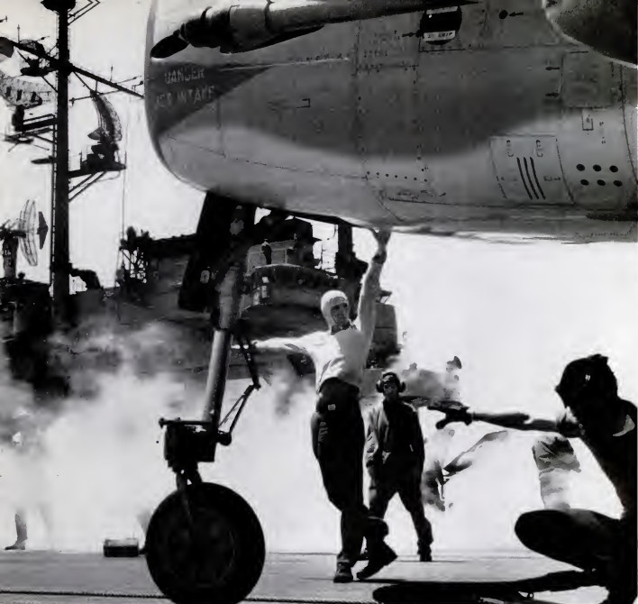
ESCAPING FROM A LAUNCHING CATAPULT, FLIGHT DECK BOSS WAVES AWAY AN F4U FIGHTER. MEN LIE ON THE DECK TO GET OUT OF THE WAY OF THE BLAST
