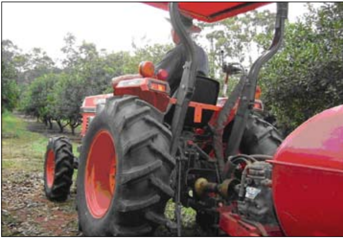
A Kubota tractor powering a macadamia orchard spray unit through the PTO at Wamuran, Queensland.
