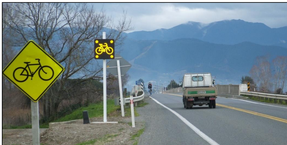
Figure 53: Inductive loop activated warning sign on Appleby bridge, SH 60, near Nelson (photo: NZTA)
