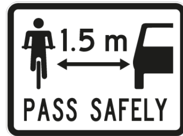
Figure 98: Pass safely sign (A43-6B TCD Rule)
