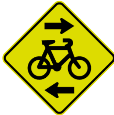
Figure 94: W16-7.1 (TCD Rule) Cycle path crossing permanent warning sign for motorists
