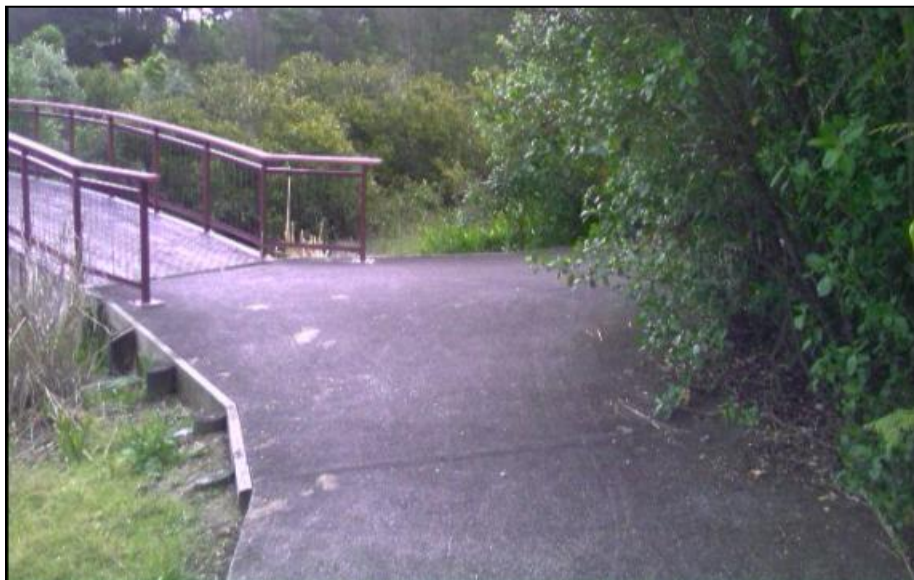
Figure 60: Poor inter-visibility at path intersection – Auckland
